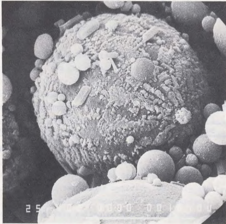
Figure 1. Electron Micrograph of Fly Ash (Magnification x 60 000)
