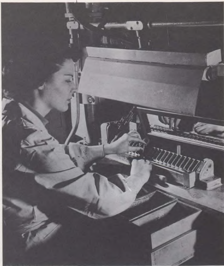
Quality control by statistical methods has proved most effective in maintaining high standards of accuracy in Canadian sporting ammunition. Here an operator checks cartridges made at a large chemical plant in Brownsburg, Quebec.
