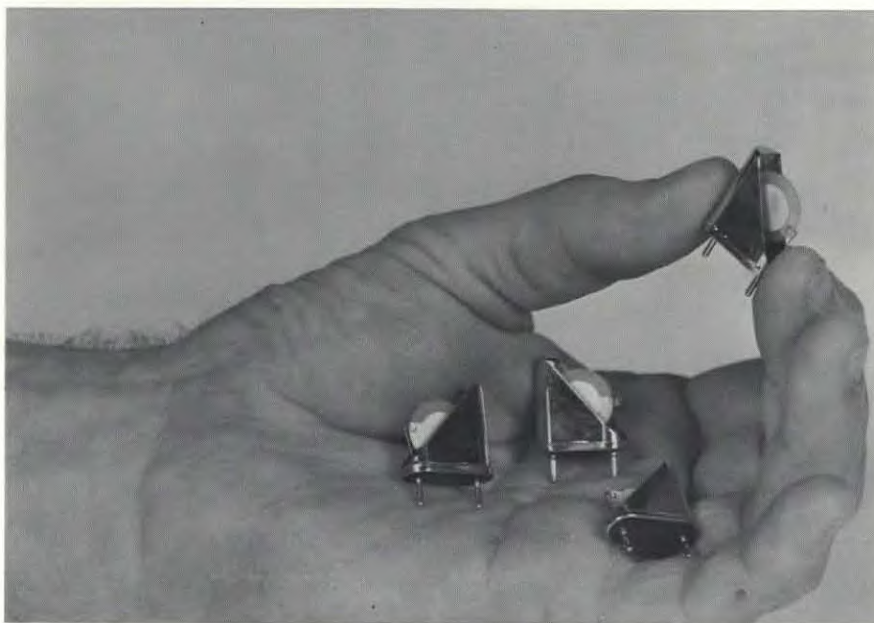
Cut-away models show Croven quartz crystals as they are set into casing to perform their electronic frequency control functions.
