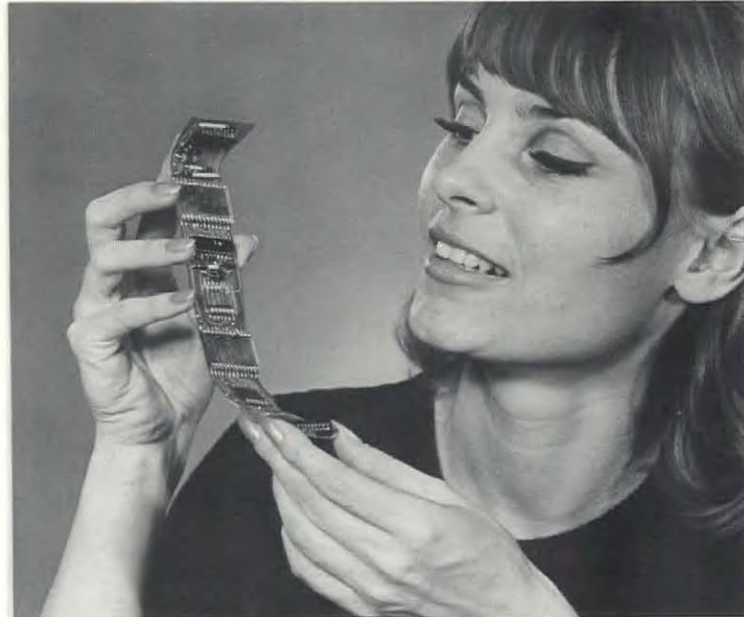
Custom designed hybrid circuit is a micro-electronic tone generator, network and tone ringer for telephones.
