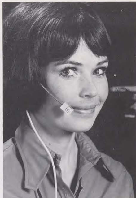
Newly developed telephone headset, weighing less than a ballpoint pen, features full-time background noise cancellation and replaces bulky headband sets in telephone, air traffic control and many other applications.
