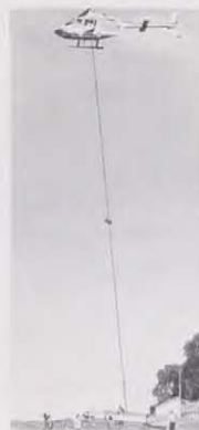
Helicopter-borne aerial geophysical electromagnetic survey equipment—one reason why Canada leads the world in this field.
