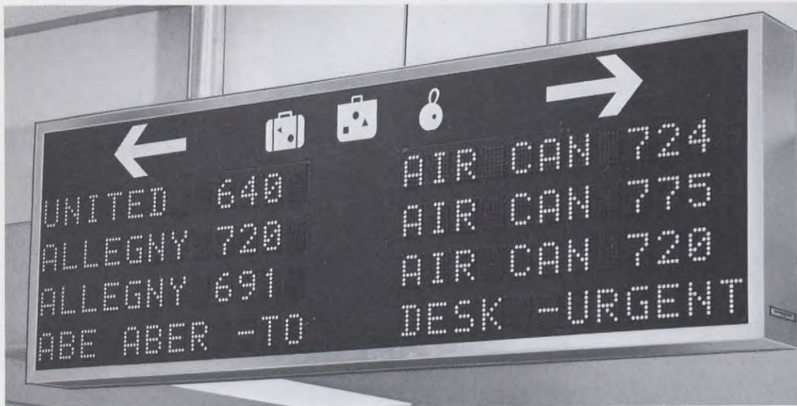
Light reflecting display components find applications in industry, transportation, financial houses, traffic displays and outdoor advertising. The electromagnetic principle of operation eliminates light bulbs resulting in very low power requirements and long life. Inherent memory retains the data displayed with ZERO POWER.
