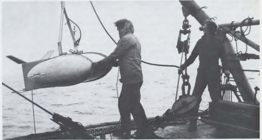
Underwater seismic system instrument package being launched in the North Sea.
