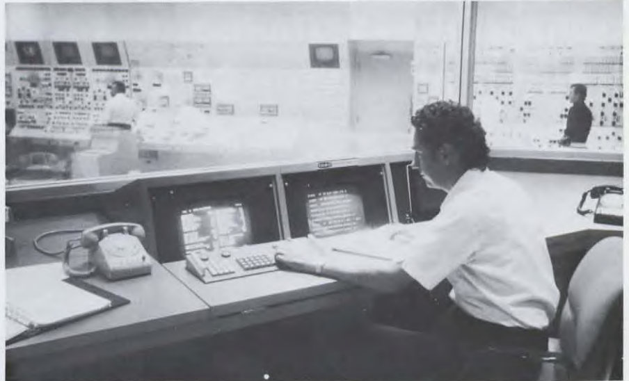
Nuclear power plant training simulator as seen from instructor's console.
