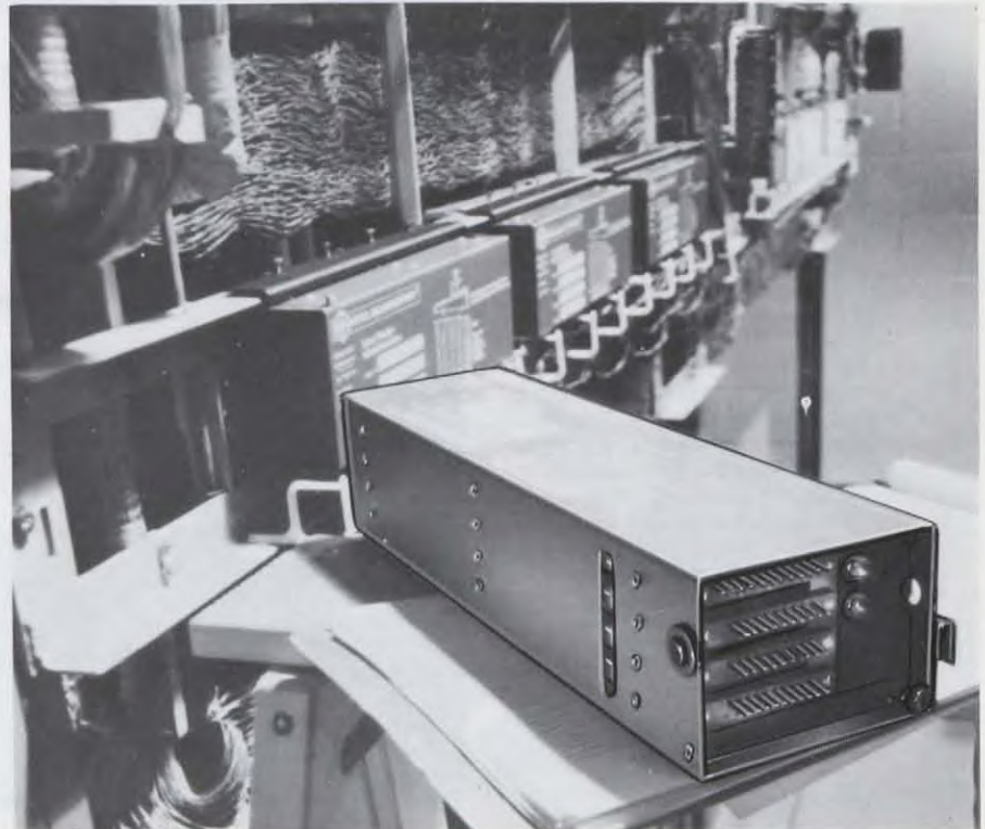
Tone to pulse telephone equipment providing an economical means of converting step-by-step offices to DTMF service.
