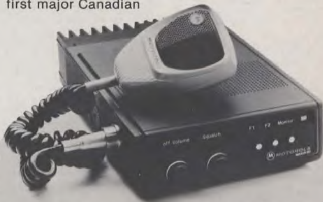
Frequency-synthesized mobile VHF transceiver.
