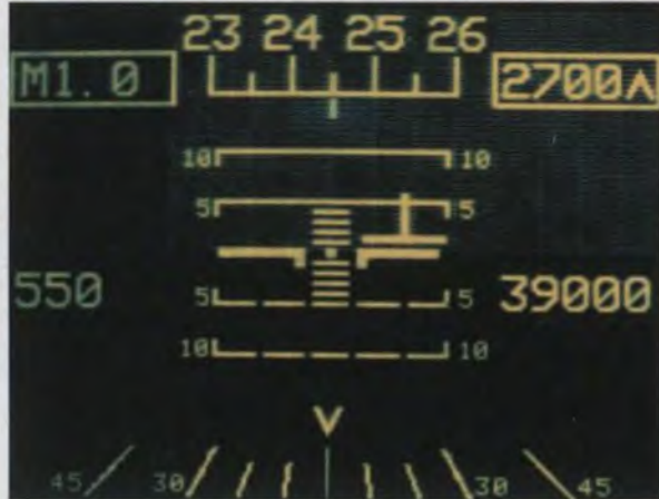
Flat panel displays, made up of large numbers of micro-miniature light emitting diodes, have been developed by Litton Systems Canada Ltd.
