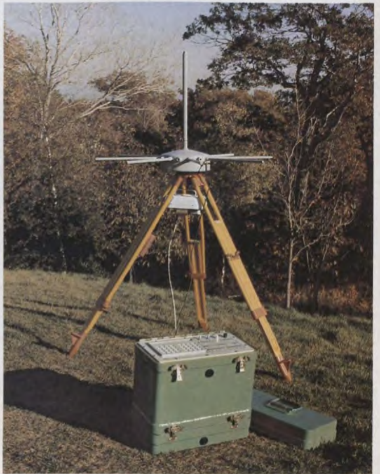
For exploration in remote areas Canadian Marconi Company makes this portable satellite navigation system which has positioning accuracy to within a few metres.
