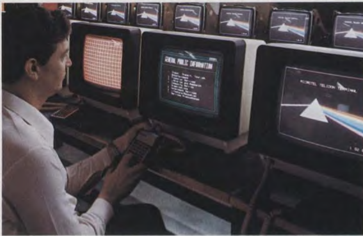
Telidon terminals under test at Viscount Industries Limited, a subsidiary of AEL Microtel.
