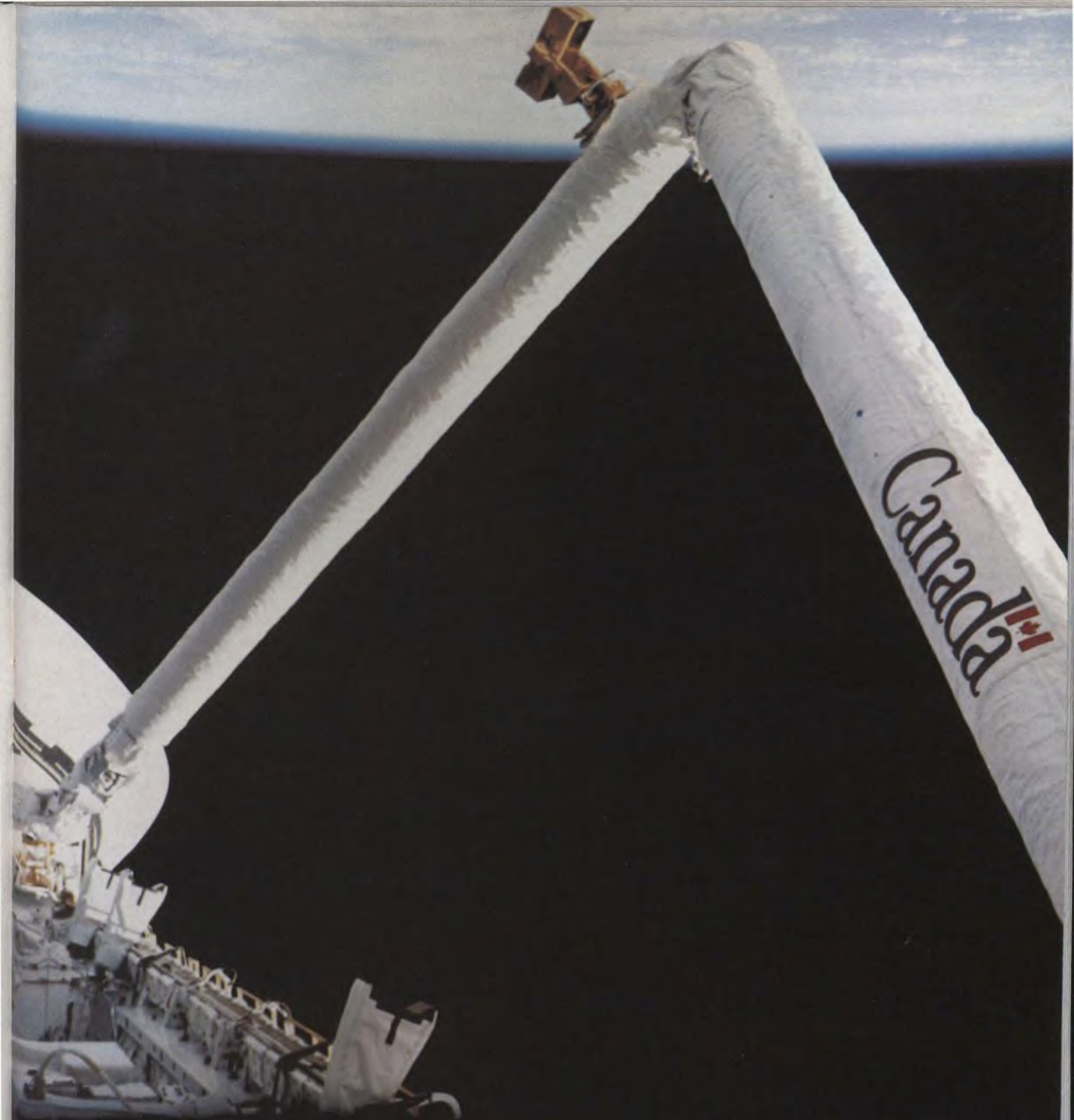
Crucial to the success of the US Space Shuttle program is the Canadian Remote Manipulator System for moving payloads from the spacecraft, shown here in space with the earth above. It was manufactured by Spar Aerospace Limited of Toronto under contract to Canada's National Research Council. The advanced robotics technology used is now being applied in other fields. Spar is the prime contractor for Canada's new Anik D satellites. (Photo NASA).
