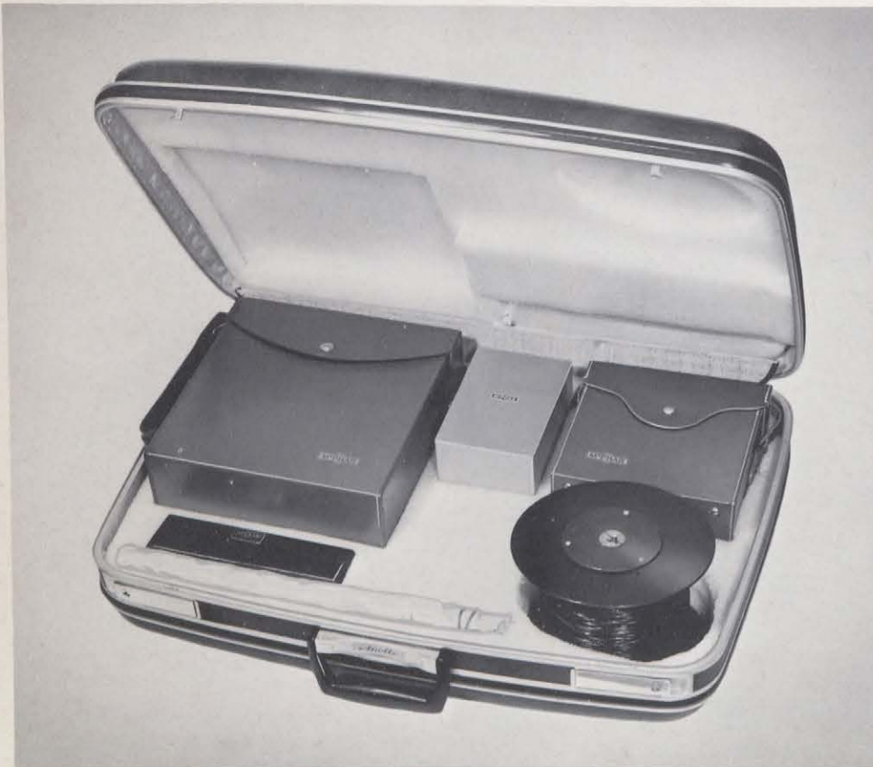
McPhar Geophysics Limited — model P670 variable frequency induced polarization system
