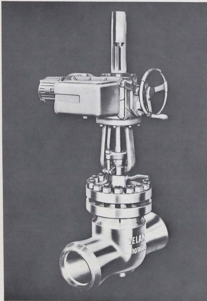
Velan Engineering Companies — 10-inch (25.4 cm) motorized nuclear valve with 1,500 psi (105 kg/cm 2 ), maximum temperature 1125°F (607°C), ANSI 1,500 pounds (680 kg). This is a primary cooling system valve for boiler isolating and primary coolant service in nuclear stations
