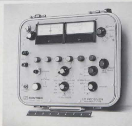
Scintrex Limited — the 2.5 kilowatt transmitter and IPR-7 Newmont type receiver of the MK VII induced polarization system
