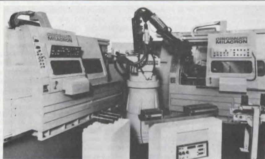
In this representative robotic production system, a Cincinnati Milacron T 3 computer-controlled industrial robot is servicing two Milacron cnc turning centers. Operations include feeding random sized parts to the machines, removing them, placing them into a laser checking gage, and then stacking them. The T 3 is the robot under development in ICAM's robotics project—Task B (see text).
