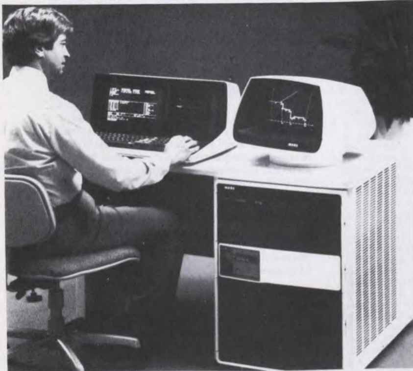
Certain NC equipment, such as MDSI's Series 300 system shown above, was designed for manufacturers with small-to-medium sized operations. The Series 300 replaces NC part programming with simplified NC part processing, so users won't have to learn a programming language.
