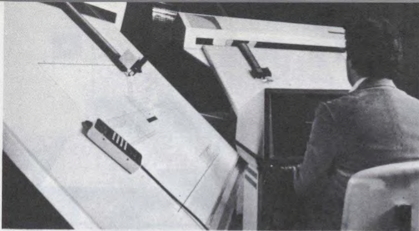
Plotter in a Data Technology system produces a drawing while the operator completes further work at the interactive terminal. The constrained-gantry digitizer behind the terminal has several lock modes for entering points on parallel lines and other restricted directions. The intelligent plotter has a built-in microprocessor-based system that removes some of the control burden from the host computer. The pushbutton hand-station placed on the plotter is for entering reference points, scaling factors, and other plotting data.
