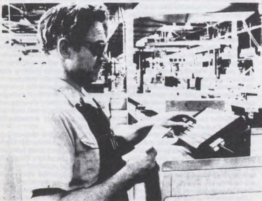
Operator assigned to repair job 'logs on' minicomputer system that helps track jobs and updates time estimates. Terminal provides prompting messages to prevent errors
