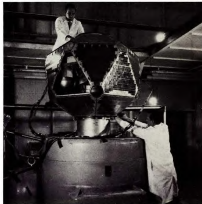
VASP Vibration Test Setup
