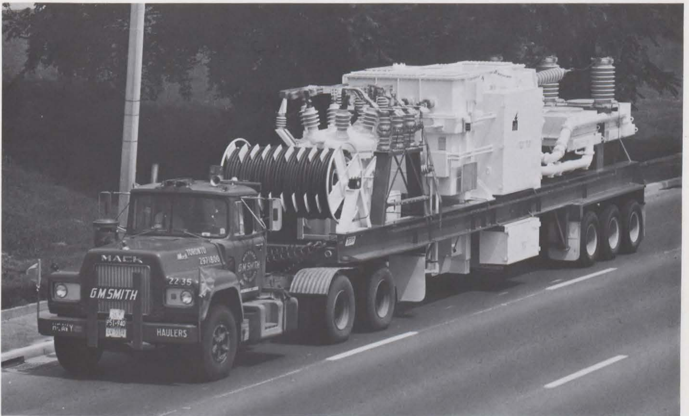
Canadian-made mobile substation recently supplied to a Venezuelan electrical utility. It is rated at 28 MVA, 3-phase, 60 Hz, 65°C rise with forced oil/forced air cooling. Primary winding is 67 kV delta connection with off-load taps. Secondary is reconnectable by an externally operated series parallel switch from 8320Y/4800 to 12470Y/7200 and has on-load tap changing. The circuit breaker has a 2000-amp continuous current rating.
