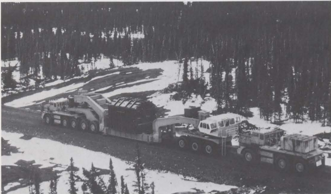
Specially developed 250 ton capacity road transporter carrying a 500 MVA, 250 kV generator transformer to the remote Churchill Falls hydro site in Labrador, Canada.
