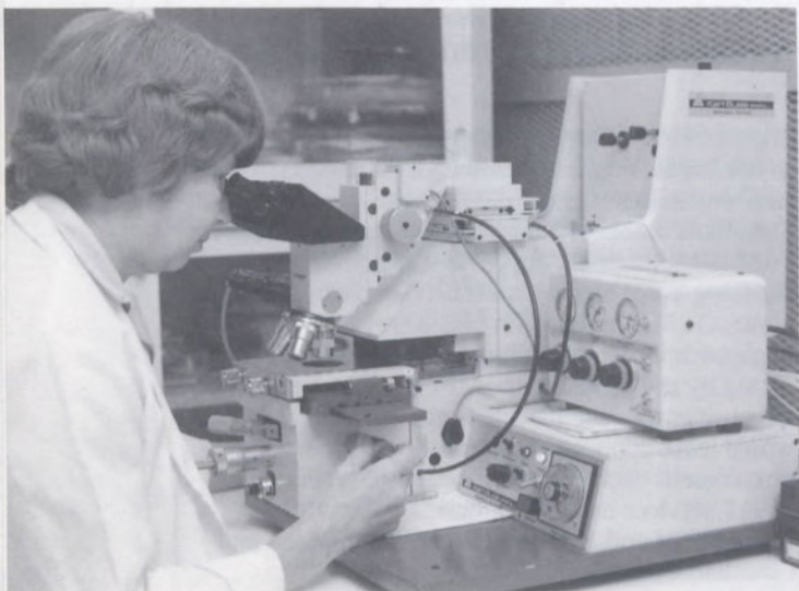
CRC technician aligning photo masks for microwave integrated circuit (MMIC) fabrication.
