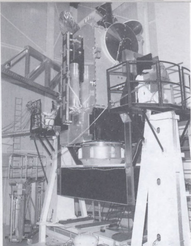
The Olympus spacecraft structural model being tested on the CRC-developed Horizontal Axis Measuring System (HAMS).
