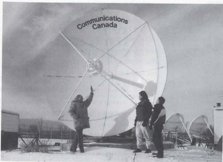
A 4.2 metre dish used in experiments for the Olympus program.
