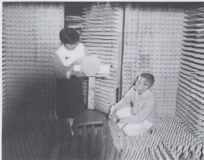
Phased-array antenna components are tested in an anechoic chamber.
