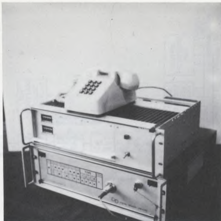
Figure 4. DAMA Controller (lower unit) and Frequency Converter (upper unit).
