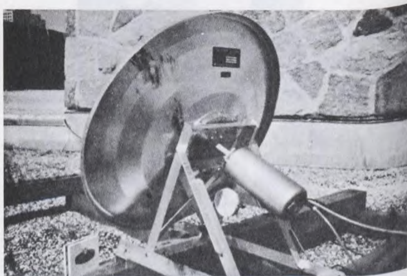
REAR VIEW, Showing down-converter unit
