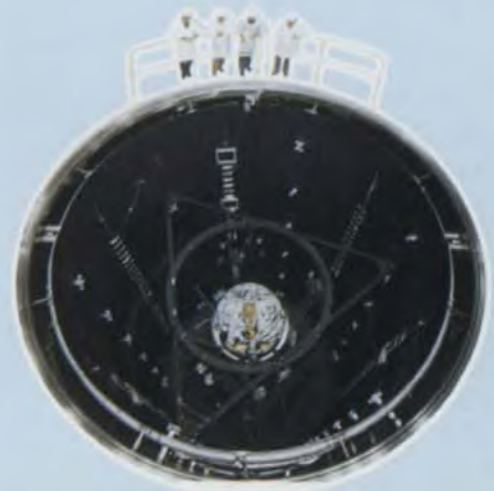
7 × 10 m thermal vacuum chamber
