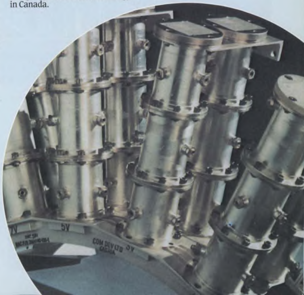
12 GHz output multiplexer/transponder
