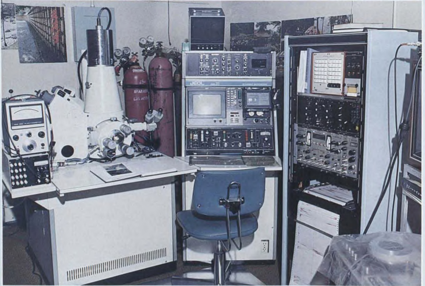
Scanning electron microscope with integral microprobe analyser
