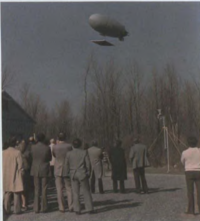
Early test of microwave power transmission to a small airship for SHARP
