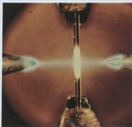
Fusing optical fibres
