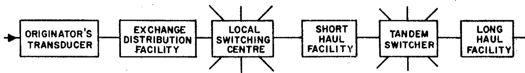
Fig. 7. Illustration of the network transmission facilities.
