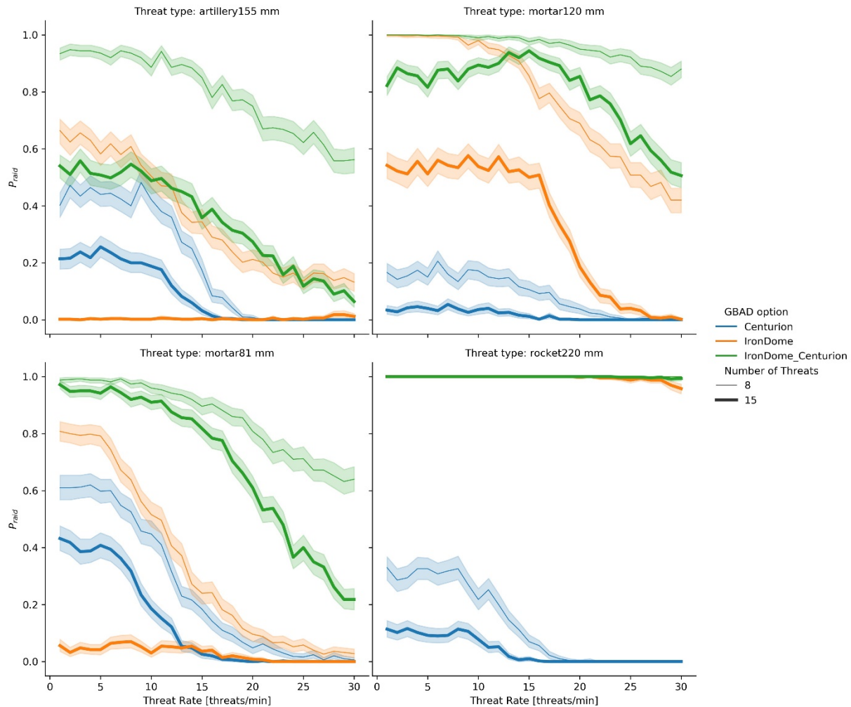
Figure 2: Probability of raid negation for scenario I (RAM threats) versus the three GBAD system options.
