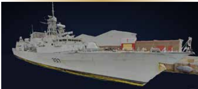
Figure 2. This 3D ship model of HMCS Fredericton was produced using more than 2,000 high-resolution 2D photos acquired by the Skydio X2D drone.
