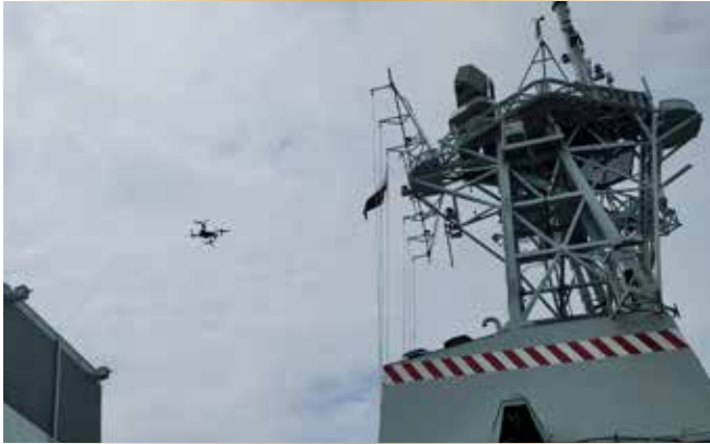
Figure 4. The hazards around a ship's structure are many, making the Skydio X2D drone's autonomous object avoidance capability a key feature of the system.
