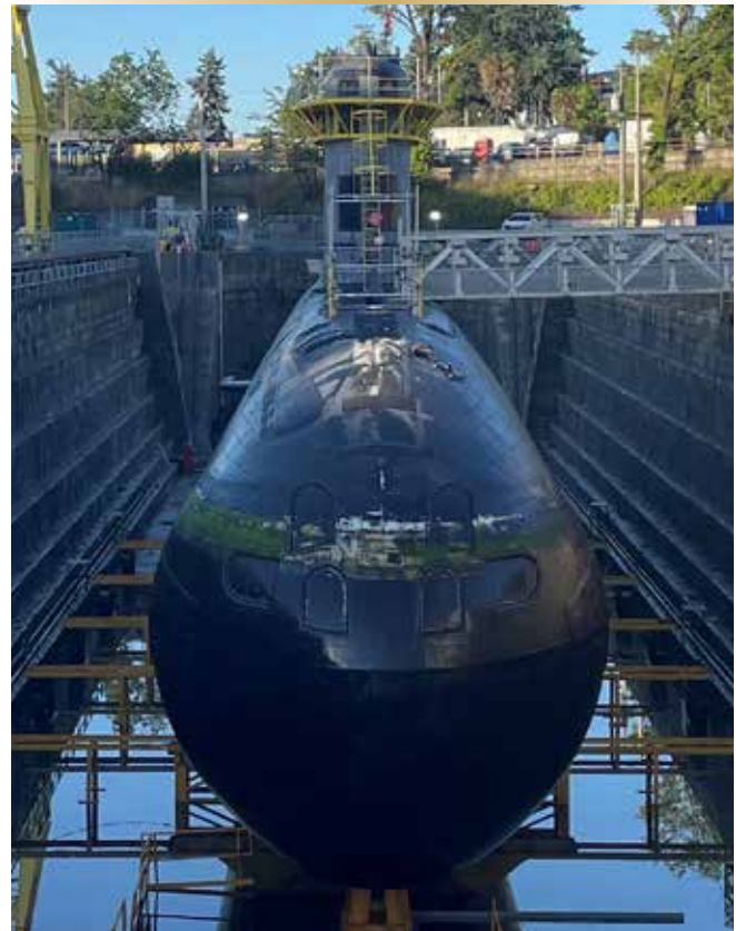
Special sliding side blocks were used to shore the submarine laterally to keep the vessel safely upright.
