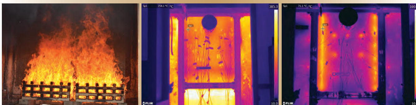
Fire at 10 minutes Ceiling temp: 290°C (550°F)
