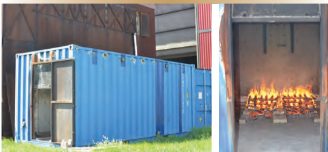
Figure 3. Bulkhead test unit external view, and the burn compartment.
