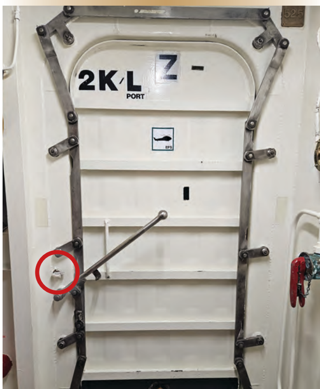
Figure 1. Quick-acting watertight door aboard a Halifax -class frigate.
