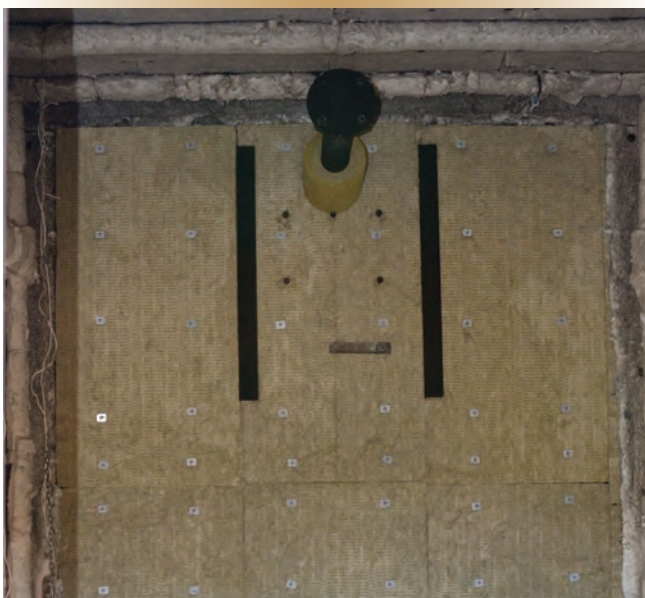
Figure 2. Rockwool A-15 insulation installed on the test bulkhead, showing exposed longitudinals, simulated door dogs and handle which were exposed to fire.
