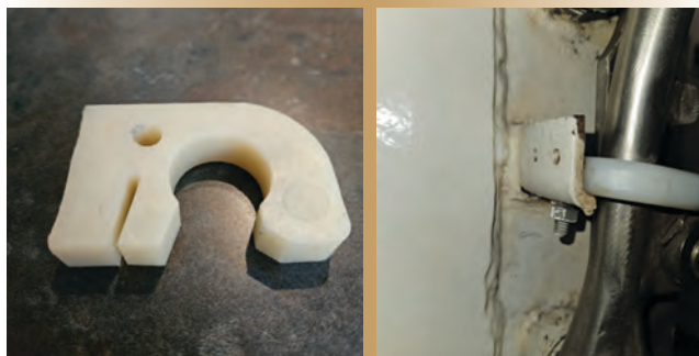
Figure 2. The polyethylene holdback currently in use.
