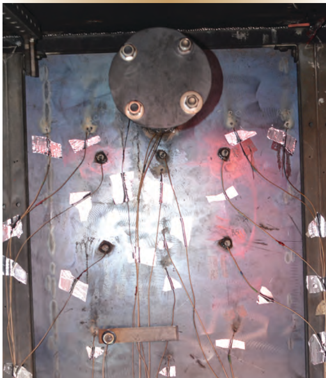
Figure 5. Thermocouples mounted on the rear of the test bulkhead.
