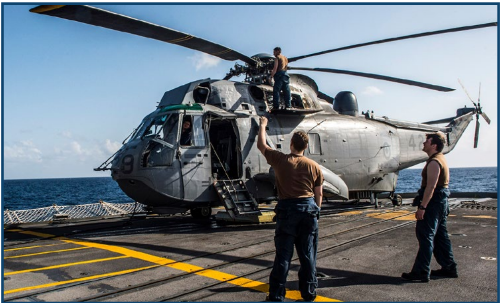
Members of HMCS ATHABASKAN air detachment perform maintenance checks on the CH-124 Sea King helicopter's rotor blades during Operation CARIBBE on May 4, 2015.
