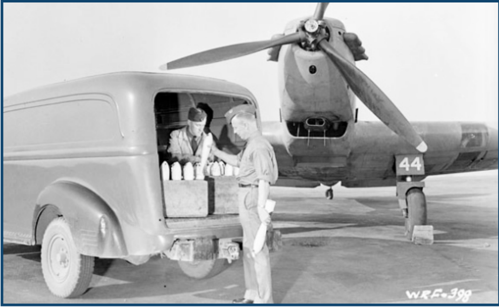
Armourers preparing to load practice bombs onto the wing racks of a Fairey Battle I aircraft at No. 1 Bombing and Gunnery School, Jarvis, ON, July 1941. The practice bombs allowed trainee bomb aimers to practise their aiming and bomb drops without the use of high explosives.
