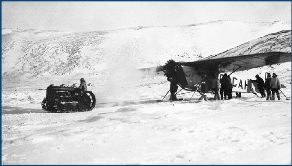
Fokker Universal "HH" being towed by a tractor during the Hudson Strait expedition. In the cold weather the oil had to be drained from the aircraft's engine and then it and the engine reheated so that the engine would turn over. The tractor was kept in a partly heated shed.
