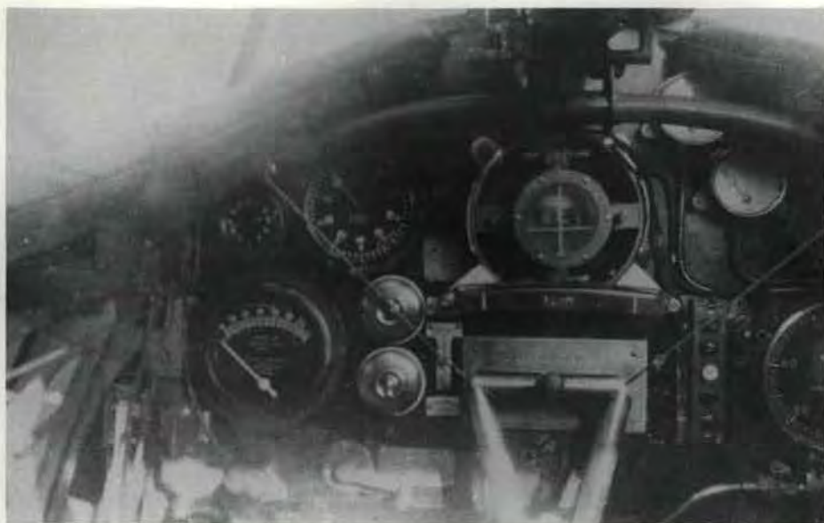
This picture of the instrument panel of the Sopwith 1½ Strutter flown by F/S/L R.F. Redpath of Montreal on the Oberndorff raid of October 1916 shows how limited were his aids to night navigation. The only relevant instruments are a compass, clock, and altimeter. (RE 20962)
