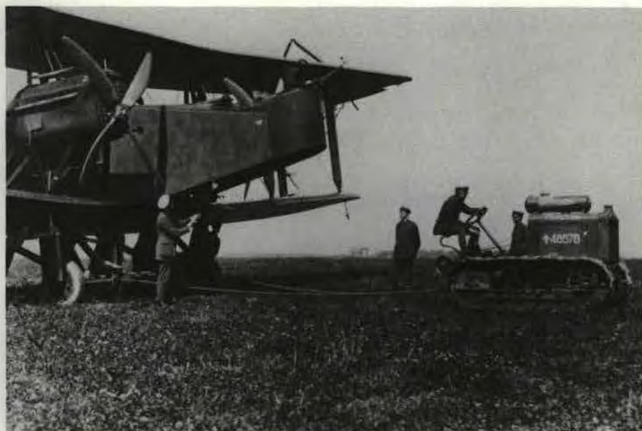
A Handley Page O/400 bomber of the Independent Force at Ligescourt, France, 29 Aug. 1918. The device below the Lewis gun in the nose is a bomb-sight: held by a safety strap the observer leaned out from his cockpit to use it. (AH 437)
