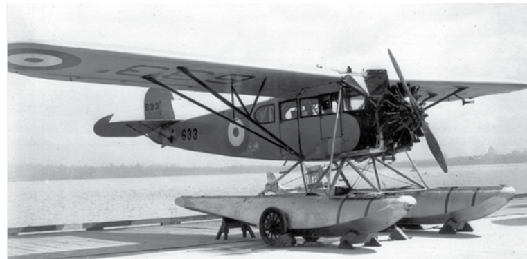
RCAF Fairchild 71 aircraft 633 is shown here, complete with floats and beaching gear, probably on Canada's West Coast. Fairchild 71B 633 (earlier G-CYVX) was one of the twelve on strength with the RCAF from 20 May 1930 to 2 October 1941, although one (G-CYVE / 630) was later converted to a 71C variant in addition to the eleven 71As. (CF photo)
