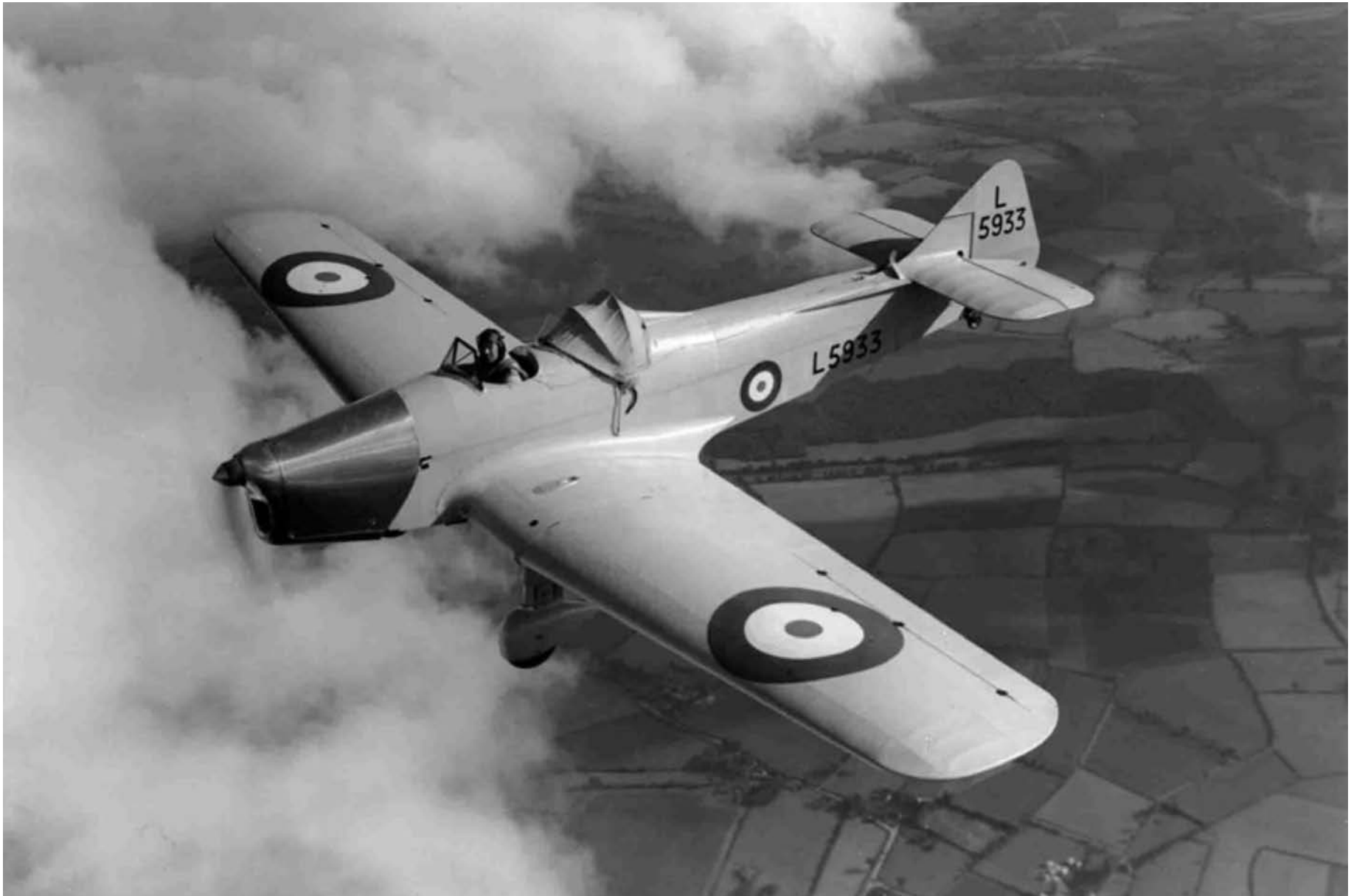
This is an image of the two-seat Miles Magister trainer used by the RAF. The second seat is under a blind-flying hood for instrument-flying-training purposes. (RAF photo)
