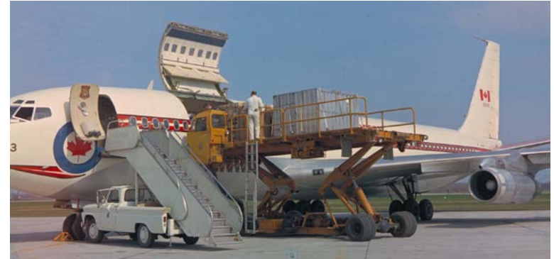
The RCAF's Boeing CC-137 served as a strategic airlifter, hauling passengers and cargo as required. The latter was facilitated by the installation of large cargo hatch doors, as seen above. (RCAF photo PCN71-268)
