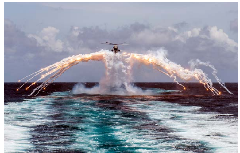
The CH-124 Sea King helicopter fleet was equipped with chaff and flare dispensers for self-defence, and this view illustrates a test of that system. (RCAF photo ET2014-7218-01)
