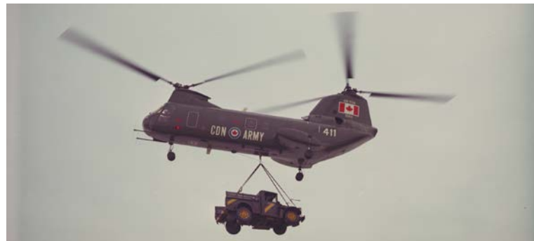
This is a CH-113 Voyageur as flown by the Canadian Army. The Army version lacked the large rear sponsons found on the CH-113 Labrador. (Canadian Army photo ZK-2054)
