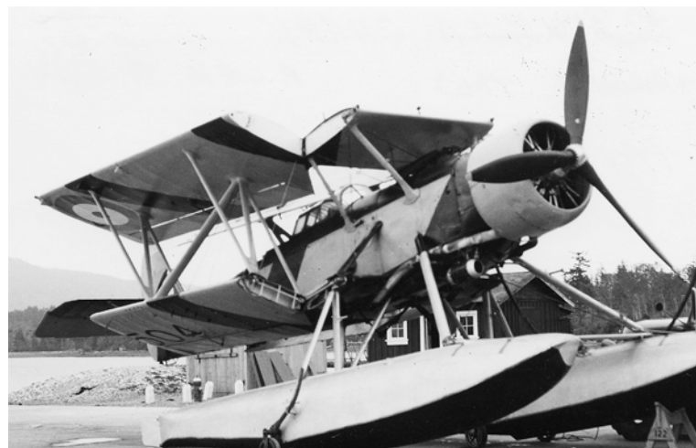
Blackburn Sharks were later used for target towing purposes, where they were given a distinctive black-and-yellow-striped paint scheme. This image also shows off the wing-fold mechanism to good effect. This is RCAF Shark Mk III (built by Boeing Canada) 504 at Patricia Bay. (RCAF photo)
