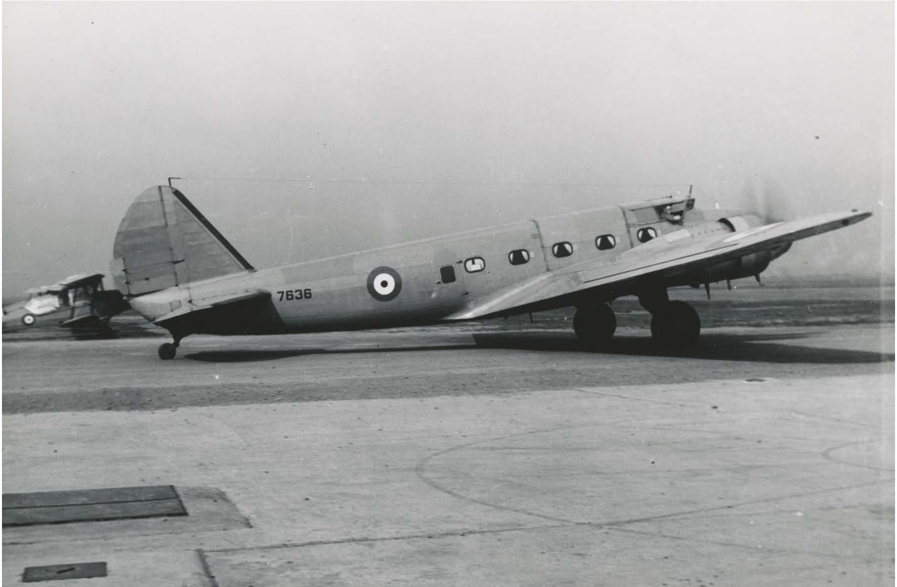
RCAF Boeing 247-D 7636 is seen here taxiing past a de Havilland Tiger Moth. Note the distinctive swept-forward cockpit windscreen used on some the aircraft. (RCAF photo)
