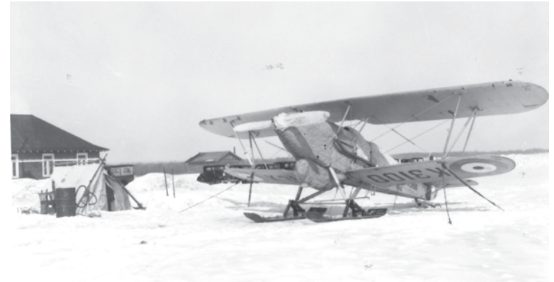
A wintry view of the streamlined Hawker Audax on skis, showing the extended exhaust and the pick-up hook underneath the fuselage. (Library and Archives Canada photo PA62981)
