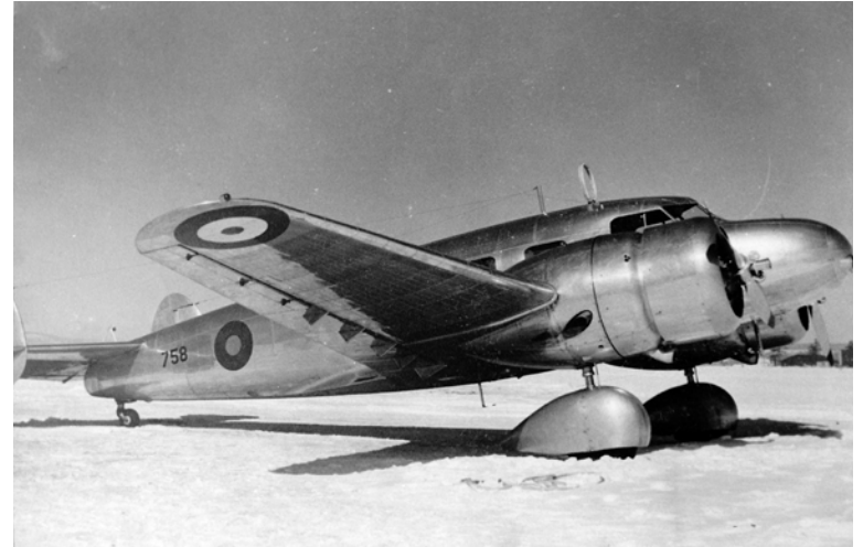
A ground view of the RCAF's Barkley Grow that illustrates its fixed landing gear. (Comox Air Force Museum photo)
