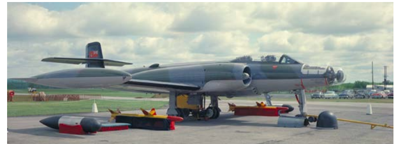
This is an interesting display of the CF-100 Mk 4B along with its possible weaponry of rockets and missiles. The radar nose cone and upper-fuselage panel have been fitted with Plexiglass replacements to allow the radar equipment to be shown. (RCAF photo PCN-418)
