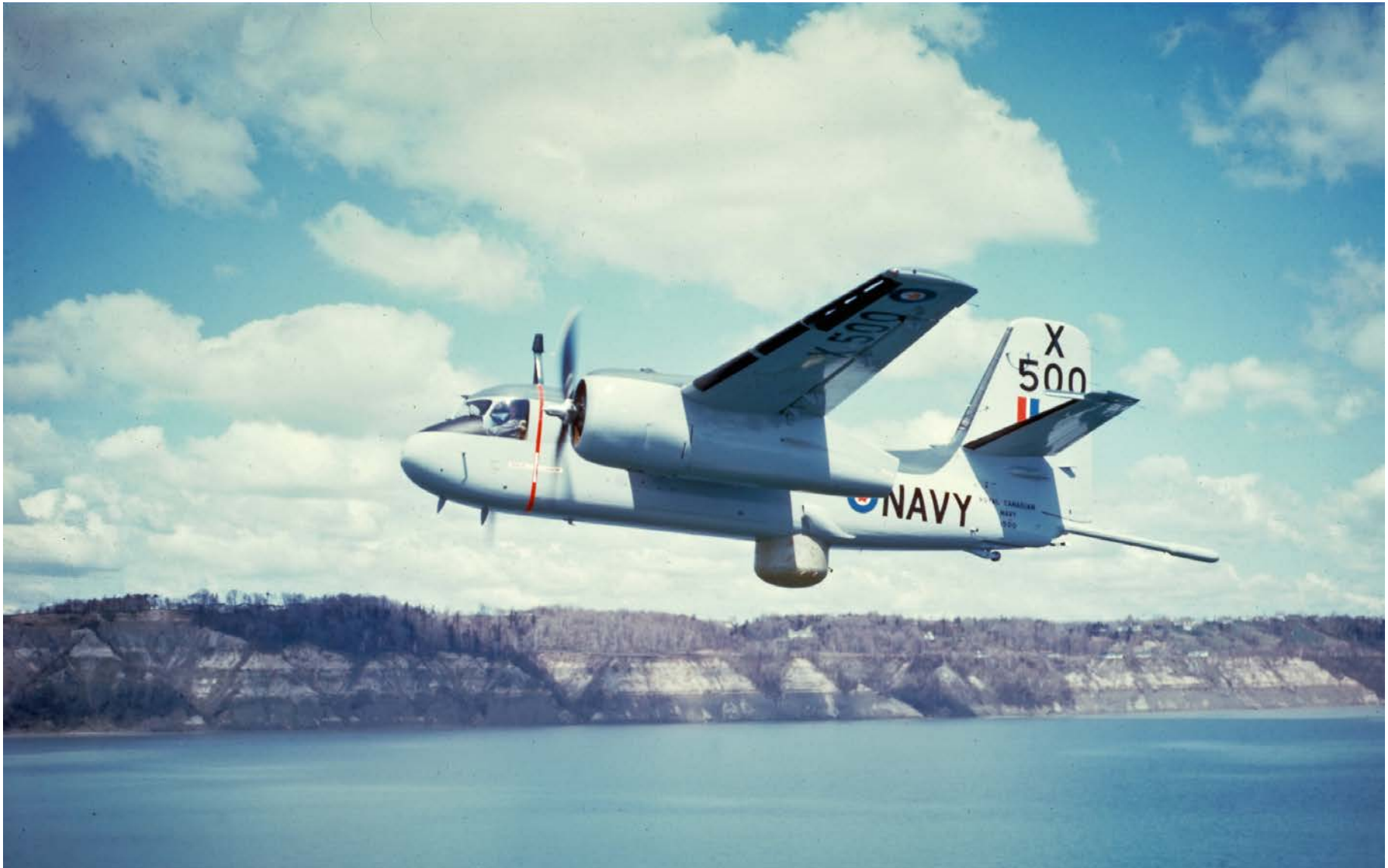
The CP-121 Tracker was designed as a carrier-borne aircraft and first served with the RCN on HMCS Bonaventure . This example from VX-10 Squadron illustrates both the lower radome and MAD boom fully deployed. (RCN photo CT-441)
