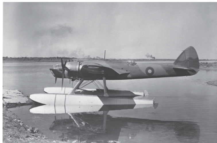
RCAF Bristol Bolingbroke No. 717 from No. 5 Squadron was tested on floats. The tests were basically successful, but no further aircraft were modified. (RCAF photo PL-140864)
