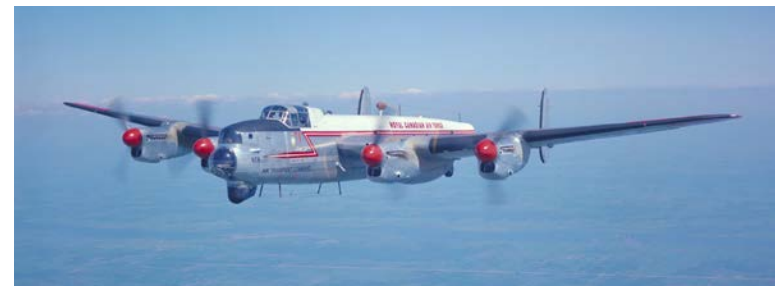
This is a heavily modified, long-nose Avro Lancaster Mk 10AR variant, no. KB976, belonging to No. 408 Squadron based at RCAF Station Rockcliffe, ON. (RCAF photo PCN-3110)
