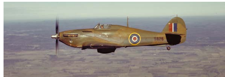
RCAF Hurricanes in Canada were often flown without the propeller spinner, giving them a very unique and distinctive appearance. (RCAF photo PC-2359)
