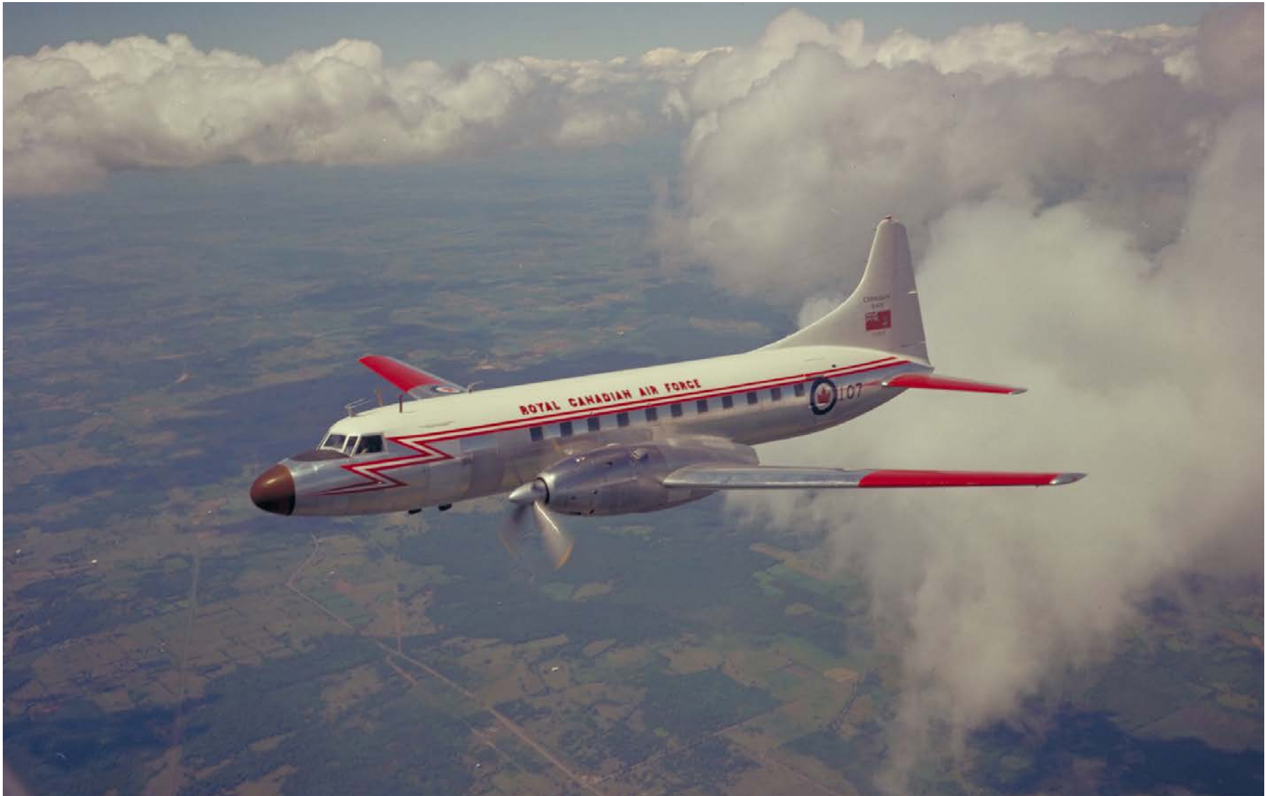
This is the CC-109 Cosmopolitan VIP transport aircraft in its revised configuration with Napier Eland 504 turboprop engines. (RCAF photo PCN-003)
