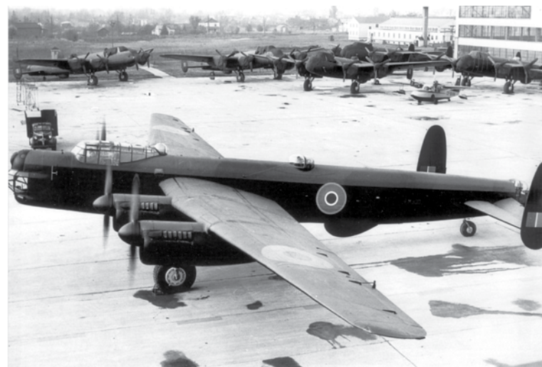
A view of the Lincoln (in this case the Canadian prototype B.Mk XV no. FM300), illustrating its overall lineage from the Lancaster, several of which are parked in the background. (CF photo)
