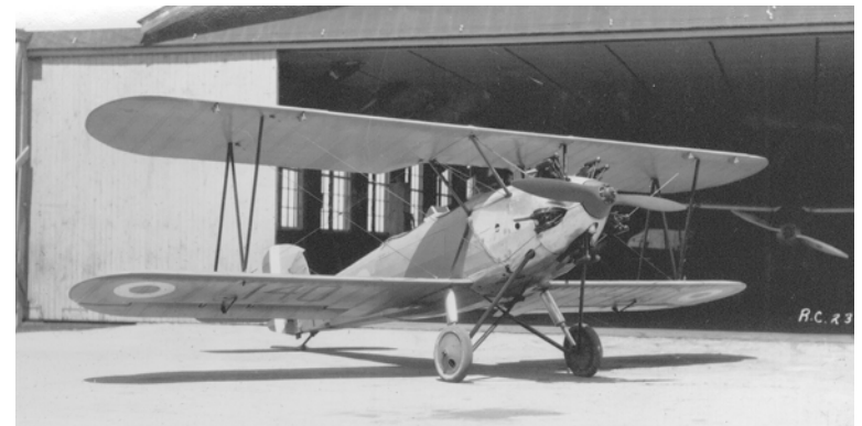
These are two views of the attractive Hawker Tomtit trainer. It possessed several features not previously seen in an elementary trainer, including Handley Page-type automatic slots fitted to the upper wings and full provision for blind-flying instruction made in the rear cockpit. (Photo courtesy of Canada Aviation and Space Museum)
