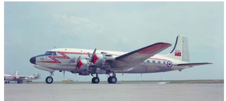
The Canadair-built C-5 was a VIP variant of the Douglas C-54/DC-4 design. It is seen here at RCAF Station Uplands on June 30, 1958. (RCAF photo PCN-433)
