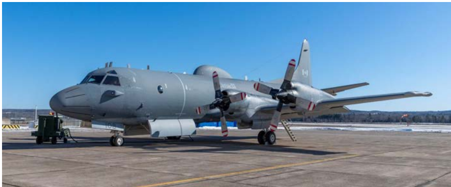
This is an example of the latest Block 4 standard of the CP-140 Aurora maritime patrol aircraft. Its external appearance has been changed considerably by the various system upgrades. (RCAF photo)
