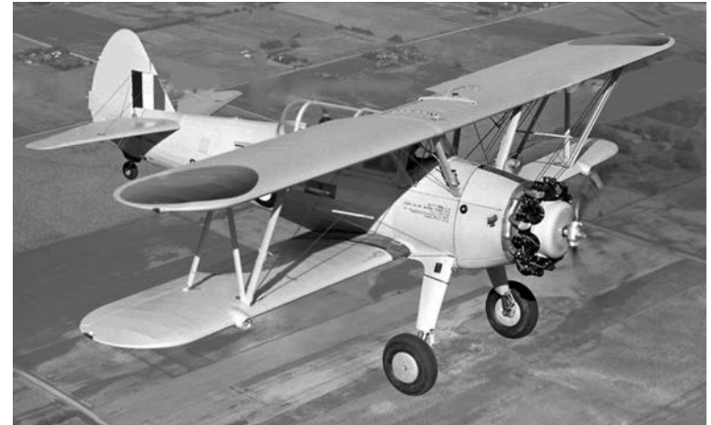
This is RCAF Stearman Kaydet FK108, which was the only aircraft ever delivered to PT-27 standard with an enclosed canopy, landing lights and other cockpit improvements. Had all the aircraft been delivered to this standard, the type might have lasted longer in RCAF service. (Photo courtesy of the Boeing Company)
