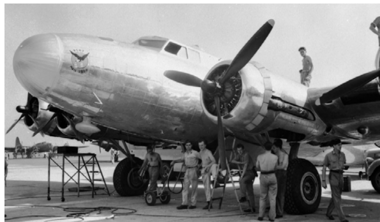
This is the RCAF's Boeing B-17 Flying Fortress 9205 in its final modified form in August 1944. It is stripped of paint to remove additional weight, with a hinged cargo nose and with other interior modifications to facilitate transport operations. (RCAF photo)
