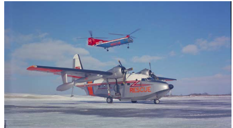
The Composite Units (KUs) within the RCAF used a mixture of helicopters along with their CSR-110. Here, a Vertol H-21 “Flying Banana” hovers over its stable-mate. The versatility of these helicopters would eventually mean the demise of the amphibian in the SAR role. (RCAF photo PCN-4344)
