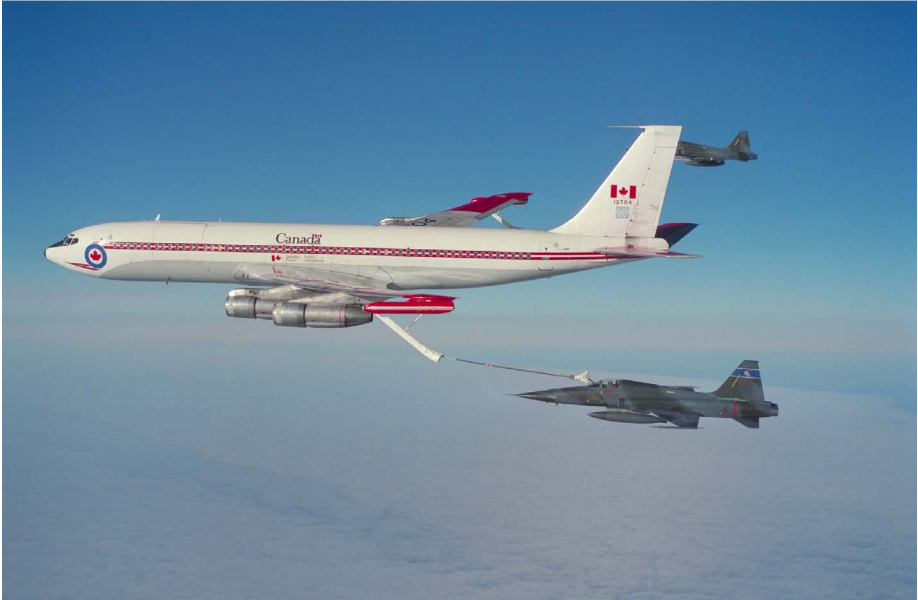
First acquired in 1970, the Boeing CC-137 served the CF both as a strategic airlifter and, as shown here, as an air-to-air refueller for up to two fighter aircraft. The CC-137 fleet was retired in the summer of 1996. (RCAF photo)
