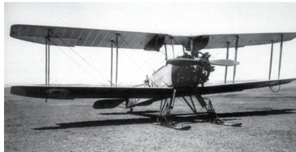
A view of the Avro Lynx with a trial ski installation for RCAF service. (CF photo)
