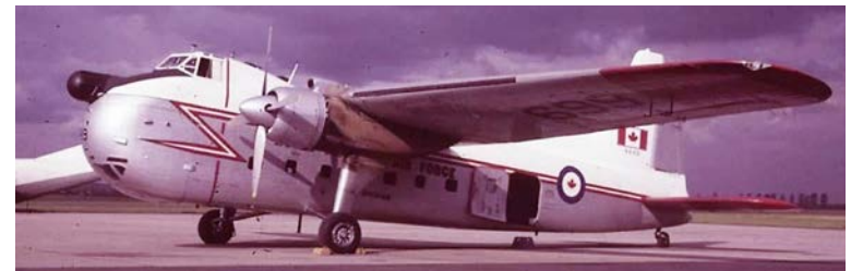
This is the RCAF Bristol Freighter in its final form, with a revised non-tactical paint scheme and weather radar added to the nose. (RCAF photo)
