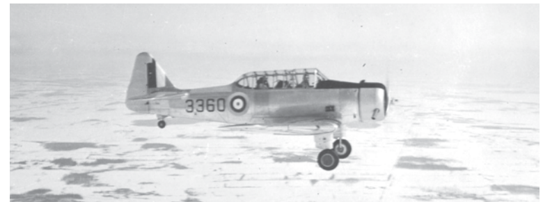
This airborne view of a Yale from No. 31 SFTS in Kingston clearly illustrates the aircraft's fixed undercarriage, which distinguished the type from its successor, the Harvard. (Photo courtesy of Stanley Leversedge)
