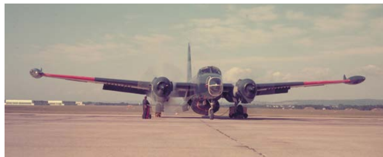
This view illustrates one of the earliest models of the RCAF Neptune. There are no J34 jet-engine pods outboard of the regular piston engines. (RCAF photo PCN-1592)
