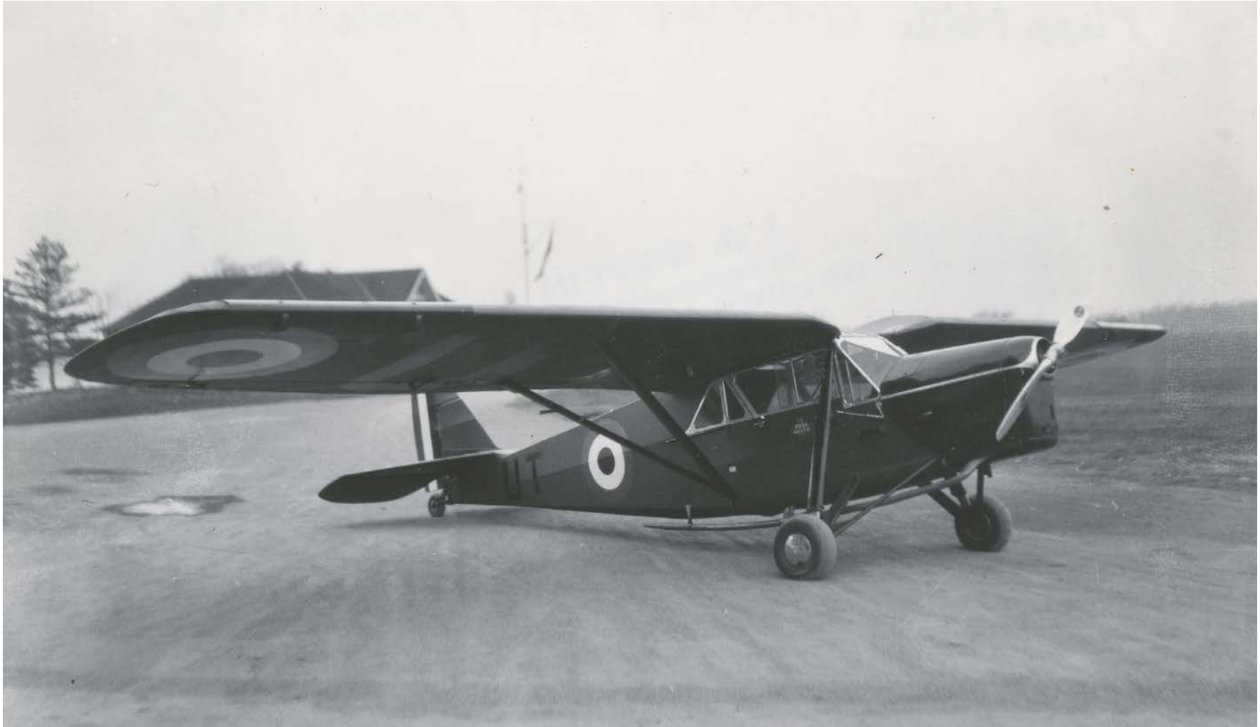
RCAF Puss Moth G-CYUT clearly displays its high-wing monoplane configuration in this photograph. (RCAF photo HC4795)
