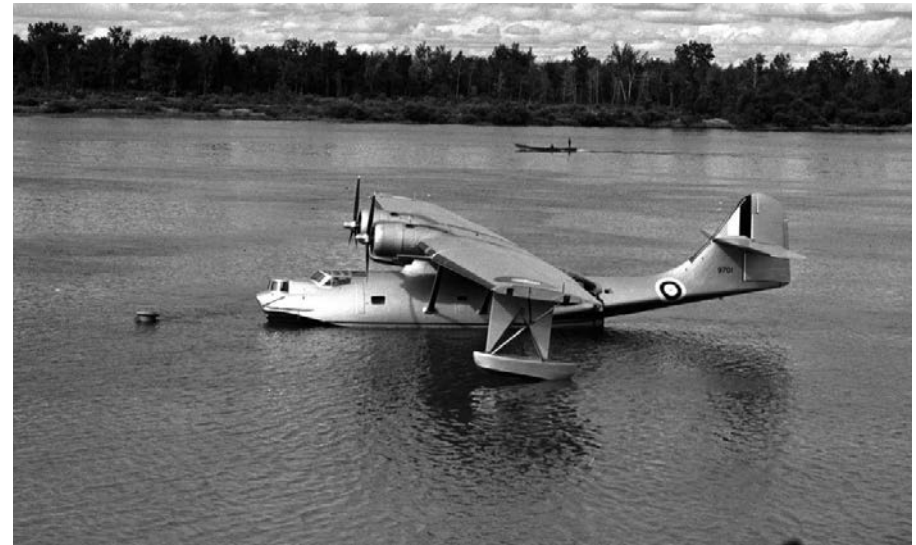
Two views of RCAF Catalinas moored on the water, the pure amphibious variant of the type. Bringing these aircraft ashore required special beaching gear or a crane. (RCAF photo and RCAF photo PL-5731)
