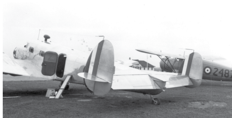
The sole RCAF Model 212, shown here, was virtually identical to the more numerous Lockheed Model 12 Electra Juniors that were also used by the service. A Norseman is in the background. (Library and Archives Canada photo PA64052)
