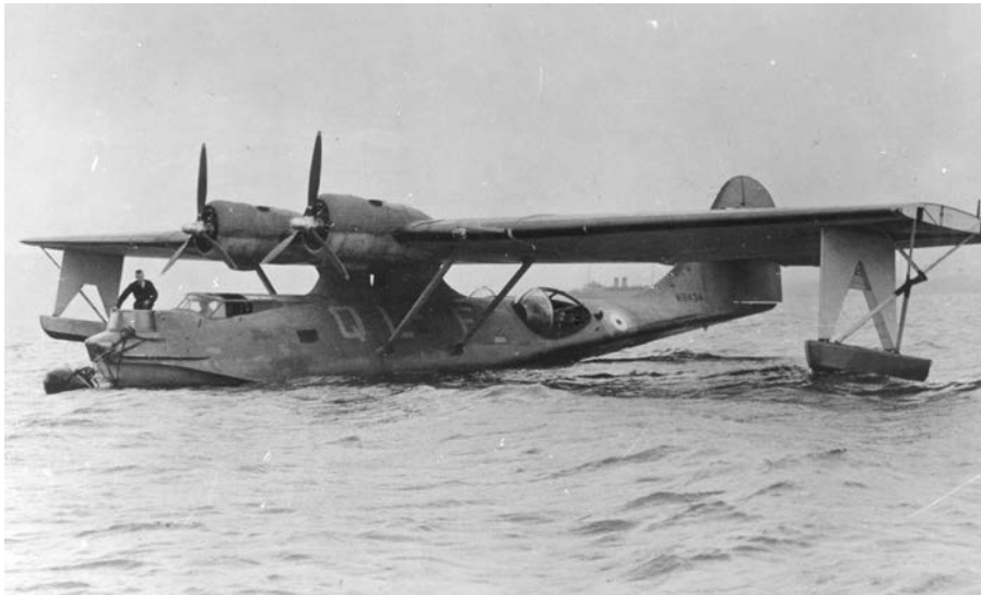
Two views of RCAF Catalinas moored on the water, the pure amphibious variant of the type. Bringing these aircraft ashore required special beaching gear or a crane. (RCAF photo and RCAF photo PL-5731)
