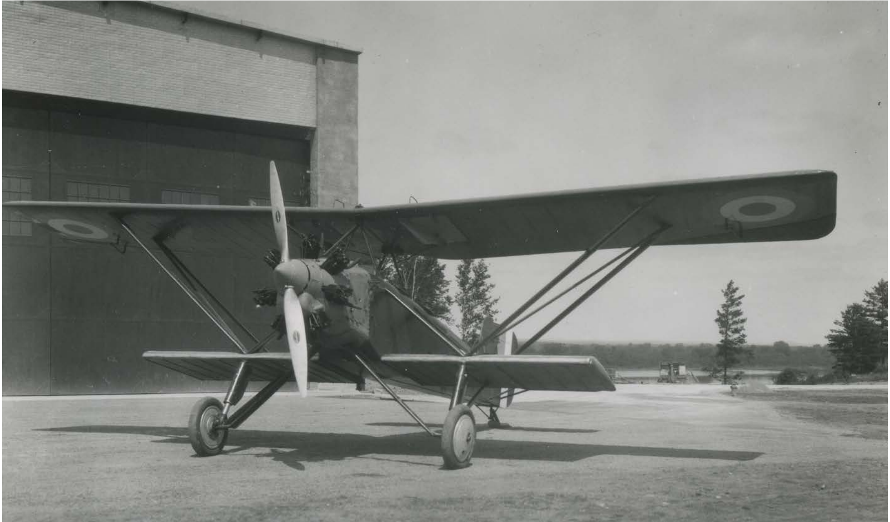
The sole Canadian Vickers Vigil G-CYZW displaying its unusual sesquiplane wing configuration. (RCAF photo HC-3046)
