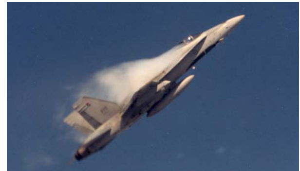
This is a view of a CF-188 Hornet in a high-alpha manoeuvre, clearly illustrating the vortex being generated off of the leading-edge extension (LEX) fence. (CF photo)
