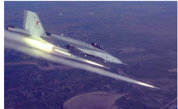
This photo illustrates a CF-188 Hornet from the Aerospace Engineering Test Establishment test firing Canadian-developed CRV7 rockets. (CF photo)
