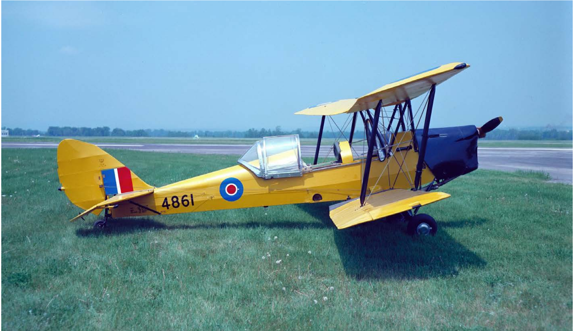
This is a view of restored RCAF Tiger Moth 4861. Note the canopy installed for Canadian winter operations. The trainer could also be operated on skis. (Canadian Forces photo)
