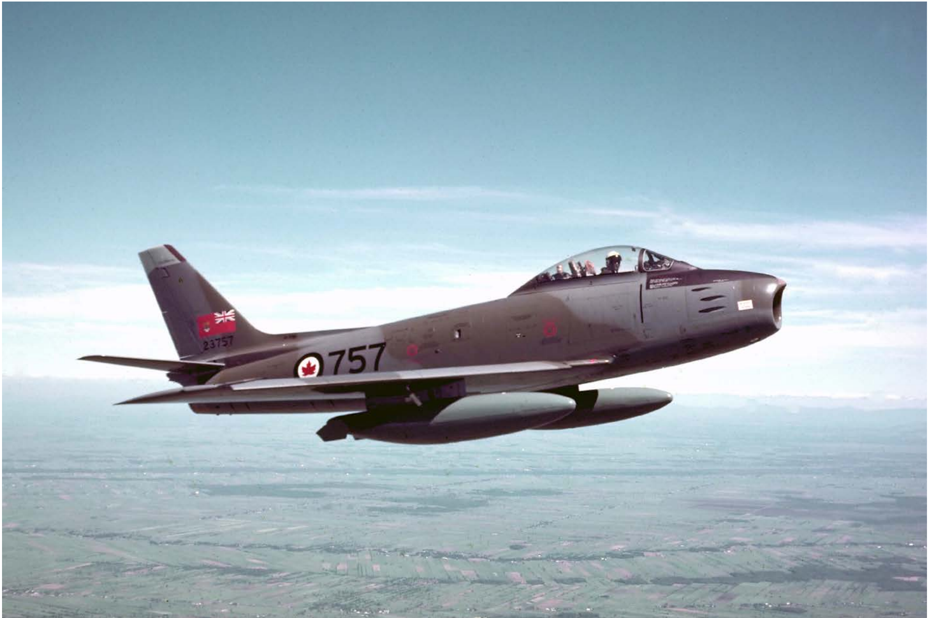
Sabre 23757 was one of 390 Canadair CL-13B Sabre Mk VI (the last version with Avro Orenda 14 engines) that served with the RCAF. This Sabre is carrying the camouflage developed for all RCAF European-based operational aircraft. The photo was taken while the aircraft belonged to No. 1 Overseas Ferry Unit (OFU) based at St-Hubert, Quebec, which was formed in 1953 to ferry Sabres and T-33s across the North Atlantic. (RCAF photo PC-2144)
