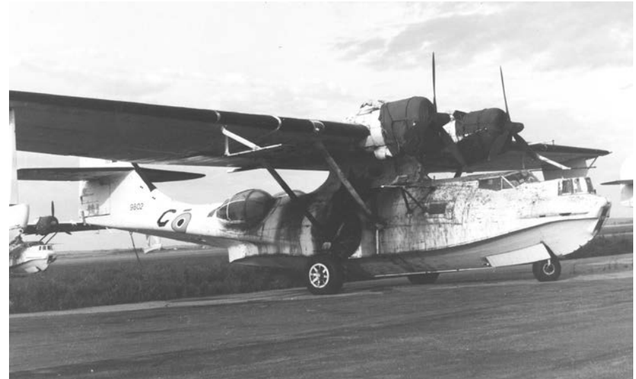
Two views of RCAF Cansos, one post-war SAR example, left, and a war-weary ASW example (as evidenced by the radar antennas under the wings) in open storage at RCAF Station Moose Jaw. (RCAF photo PC-1606 & T. F. J. Leversedge Collection)
