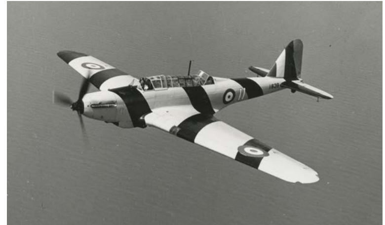
This is a fine study of the Fairey Battle aircraft—in this case, a colourfully marked target-towing aircraft with yellow and black stripes. (RCAF photo WRF334)
