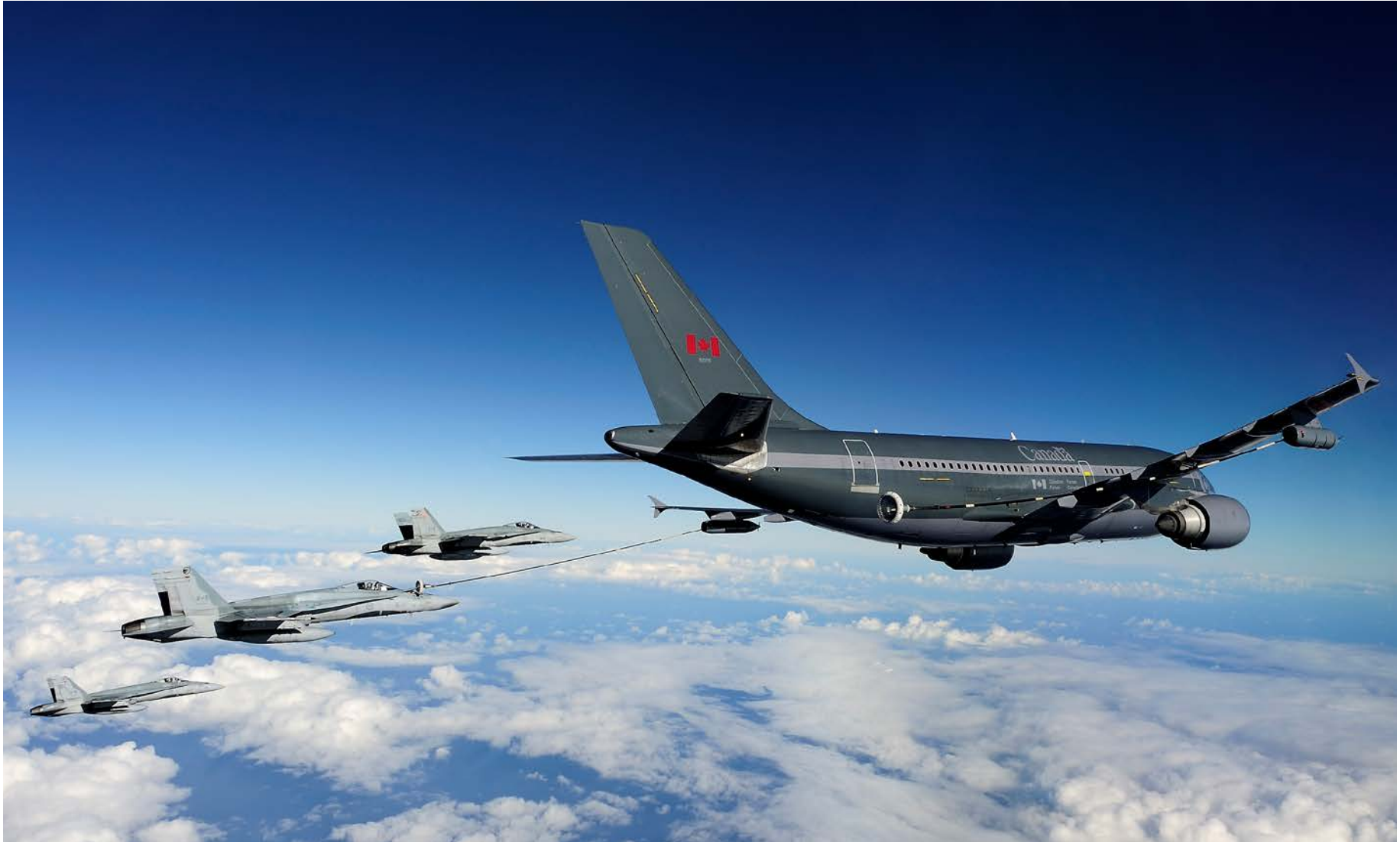
CC-150 Polaris A/C from 437 Transport Squadron. Originally delivered in a 194-seat passenger configuration, four of the A/C have now been modified into a combi configuration that includes the addition of a large cargo door. A removable bulkhead provides a compartment for 60 passengers in the back of the A/C and for freight, which is loaded in the front. (CF photo)
