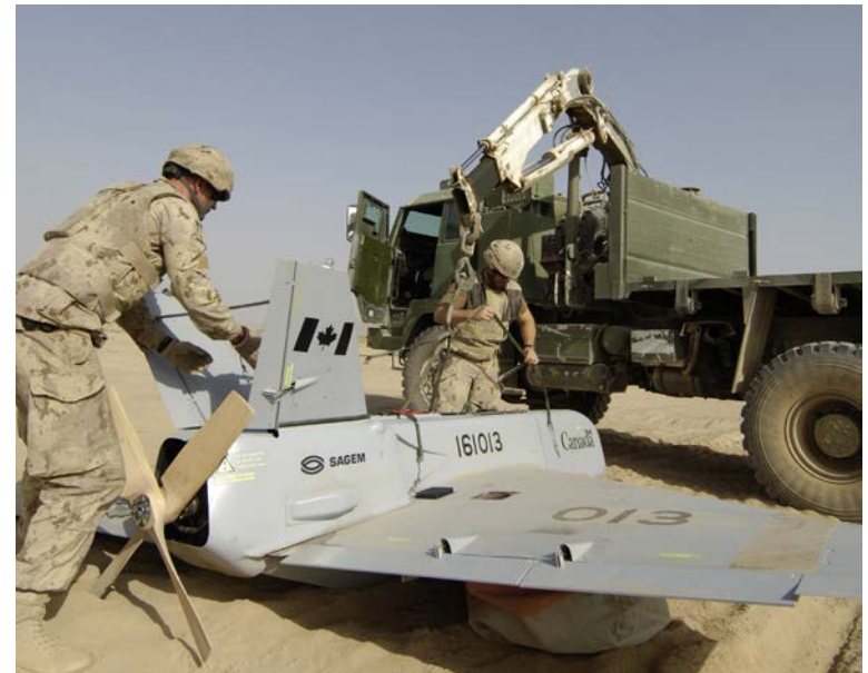
One of the CU-161 Sperwer UAVs is seen here being recovered after completing a mission in Afghanistan. (CF photo IS2006-0280[1])
