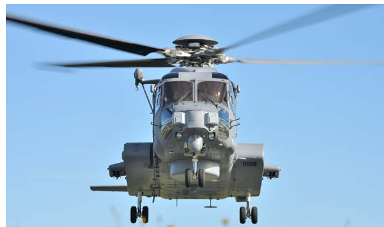
The CH-148 Cyclone possesses a wide array of sophisticated sensor systems including missile defence and forward-looking infrared camera sensors, some of which are visible on the nose in this photo. (RCAF photo SW2013-0348-16)
