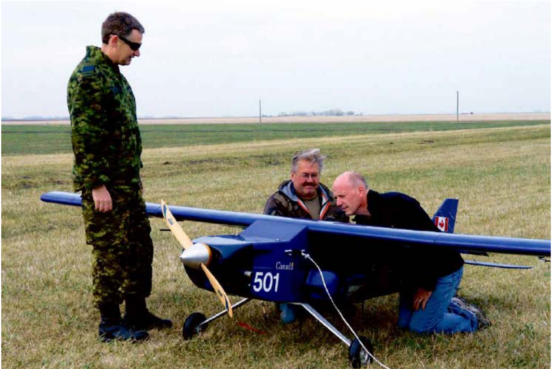
The CU-171 BTE Super Hauler was a surrogate UAS used for operational test and evaluation purposes at the Canadian Forces School of Aerospace Studies. It is shown here being trouble-shot after a mission. (CF photo)
