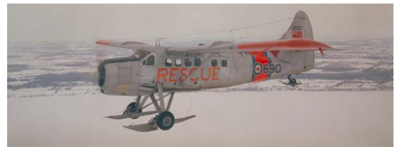
The CSR-123 Otter utility transport aircraft could be flown on wheels, skis or as a floatplane. These photos illustrate the type in all three configurations. (RCAF photos PC-211, RT118, and PCN-79-182)
