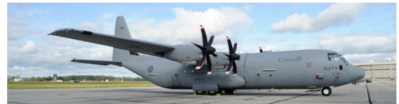
The CC-130J Hercules is a significantly redesigned aircraft with only a small percentage of things in common with the other Hercules in the CF transport fleet. Externally almost identical to its older cousins (except for 6-bladed propellers), internally it is almost completely redesigned with all-new avionics, fly-by-wire and improved cockpit controls. (CF photo FA2011-0041-18)
