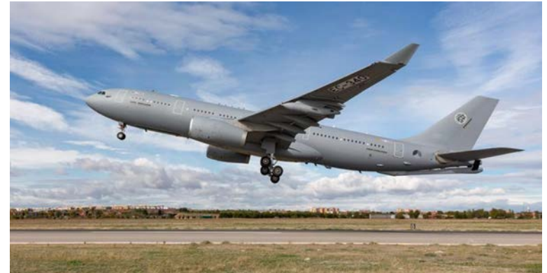
Based on the successful Airbus A330-200 commercial passenger airliner, the A330 MRTT is the military variant adapted to strategic transport and AAR capabilities. This example is an A330 MRTT belonging to the Royal Netherlands Air Force. (Photo courtesy of Airbus Defence and Space)
