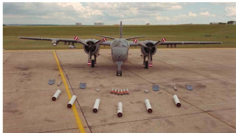
This photo illustrates some of the armament the CP-121 could carry—in this case, six LAU-5002 rocket pods with their CRV7 rockets. (CF photo)
