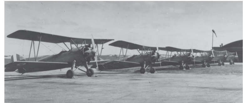
Two RCAF Avro Tutors following conversion to the army cooperation training role, as evidenced by the long hook under the fuselages. (CF photo)
