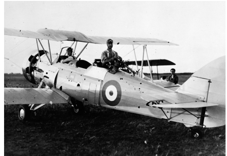
Avro 626 trainer no. 266 from No. 112 (AC) Sqn is seen here prior to departing on a mission exercise. The observer/gunner is holding a flexible Lewis machine gun. (RCAF photo PMR76-588)
