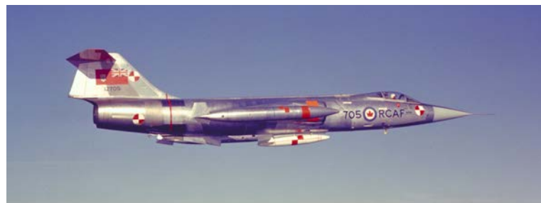
CF-104 Starfighter 12705 from the Central Experimental and Proving Establishment is seen here in a rare photo carrying the inert ballistic shape of a nuclear bomb in April 1964. The circular red-and-white markings were added to the weapon and the aircraft to aid tracking cameras. (RCAF photo PCN-5408)
