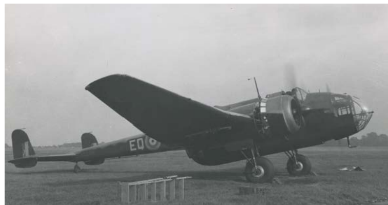
This Handley Page Hampden, AE288, belonged to No. 408 Sqn. The aircraft is apparently receiving a ground engine run-up, as evidenced by the missing engine cowling panels. (RCAF photo PL-4715)
