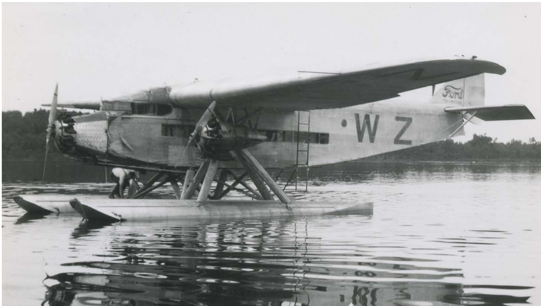
In RCAF service, the Ford Trimotor was flown on wheels, skis or floats, the latter shown in this photo. (RCAF photo HC3043)
