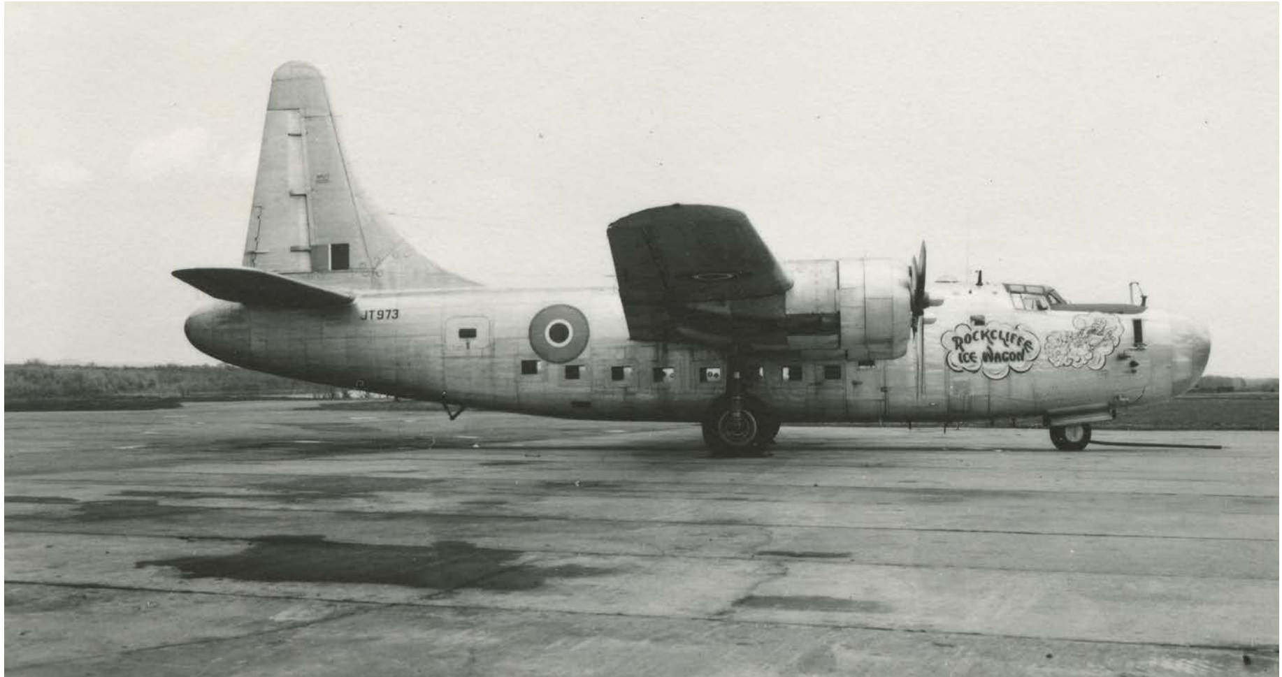
The Consolidated RY-3 Privateer loaned by the RAF became the basis of the first RCAF "Rockcliffe Ice Wagon," which was used for early experiments in aircraft icing and de-icing trials. (RCAF photo via the Jack McNulty Collection)
