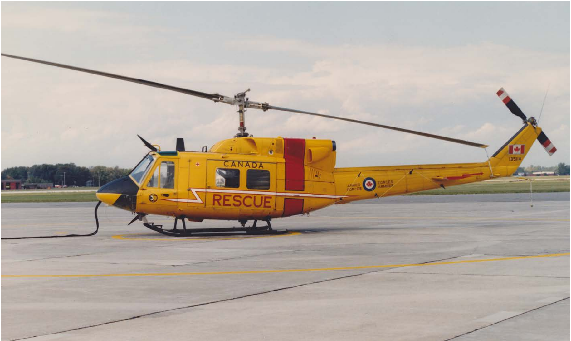
The CH-135 Twin Huey was also operated in the search and rescue role. This example also is equipped with the Canadian-developed Wire Strike Protection System (WSPS), which consists of wire cutter blades mounted above and below the windscreen. (CF photo PCN 82-121)
