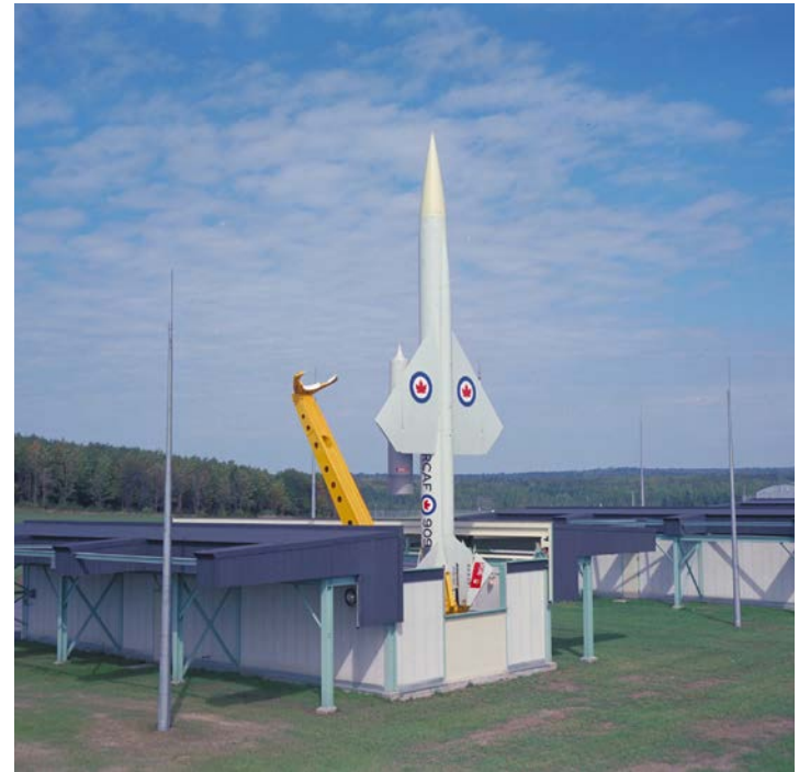
Above: This view illustrates the BOMARC missile stowed in its hangar. Below: The missile has now been erected for launch and the erection arm is retracting. (RCAF Photos PCN-4077 and CPN-4083)
