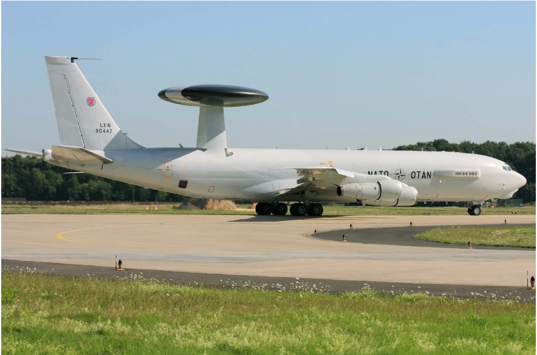
The NATO version of the E-3 Sentry. (Photo courtesy of Jean-Marie Hanon)
