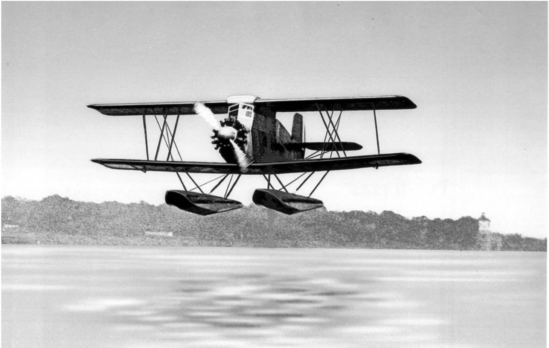
The inspiration behind the design for the Vickers Vanessa was a Stinson enclosed-cabin biplane, which was produced in the US. One feature the Canadian Vickers chief engineer did not like about the Stinson was the usual wire bracing for biplanes, which interfered with easy cabin access. Consequently, he introduced a system of interplane struts as clearly seen in the above photo. (RCAF photo)
