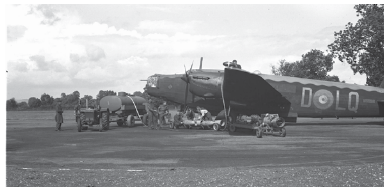
RCAF Wellington Mk II W5553 from No. 405 Sqn is shown here being bombed up and fuelled up in preparation for a mission. (RCAF photo PL-4051)
