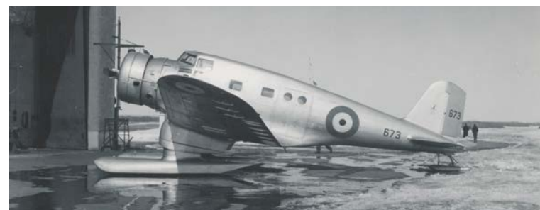
The Northrop Delta was a versatile aircraft that could be flown on wheels, floats or skis. This view of RCAF Delta 673 illustrates the ski configuration. This aircraft created the first RCAF casualties of the Second World War when it went missing on a deployment flight from Ottawa to Sidney, NS, on 14 September 1939. The wreckage was not discovered for 19 years and the crew was never found. (RCAF photo HC-8541)
