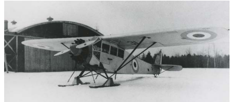
RCAF Fairchild Razorback 31 is seen here on skis. The triangular rear fuselage is evident in this photo. (RCAF photo courtesy of the Griffin Library Collection)
