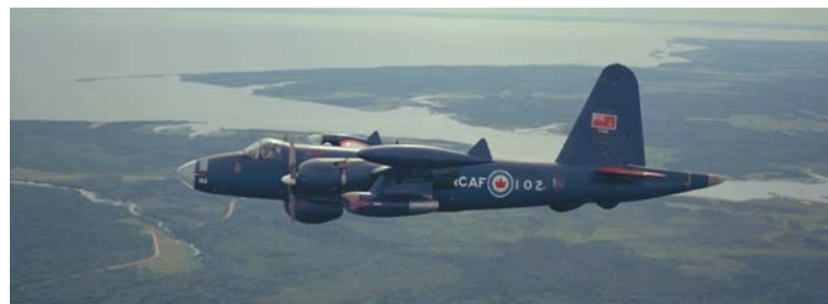
In this view of RCAF Neptune 24102, the J34 jet-engine pods are clearly visible on the outboard wing. (RCAF photo PCN-1885)
