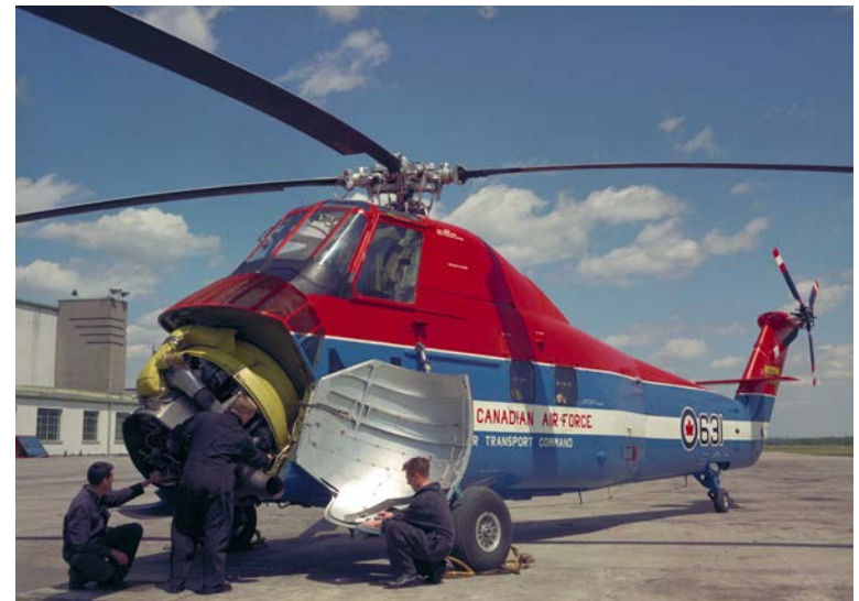
RCAF H-34 9631 is shown here receiving some maintenance attention to the radial engine. The large clam-shell front doors provided easy access. (RCAF photo)
