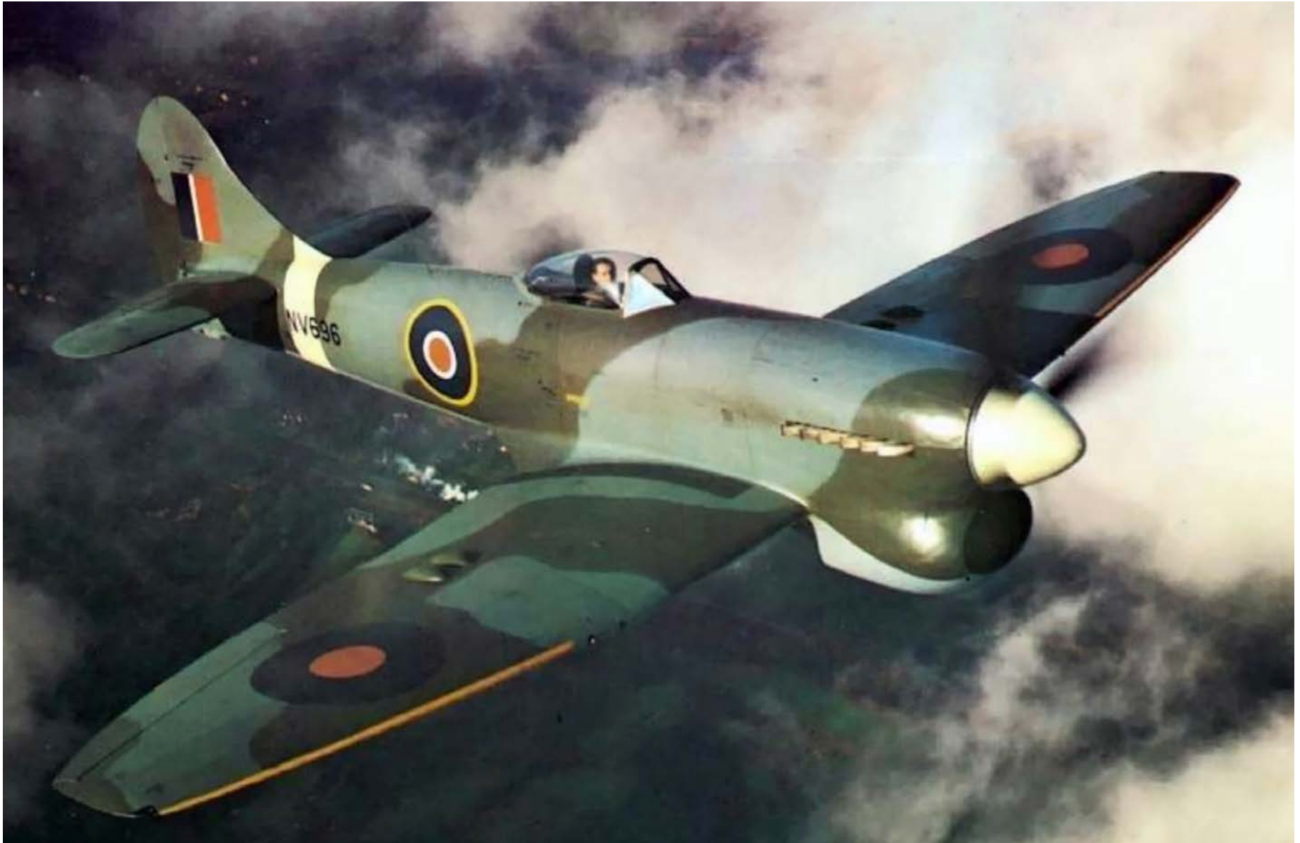
This is view of a late-model Hawker Tempest Mk V illustrating its Typhoon heritage with its distinctive "blown" canopy and nose (chin)-mounted radiator. (RAF photo)
