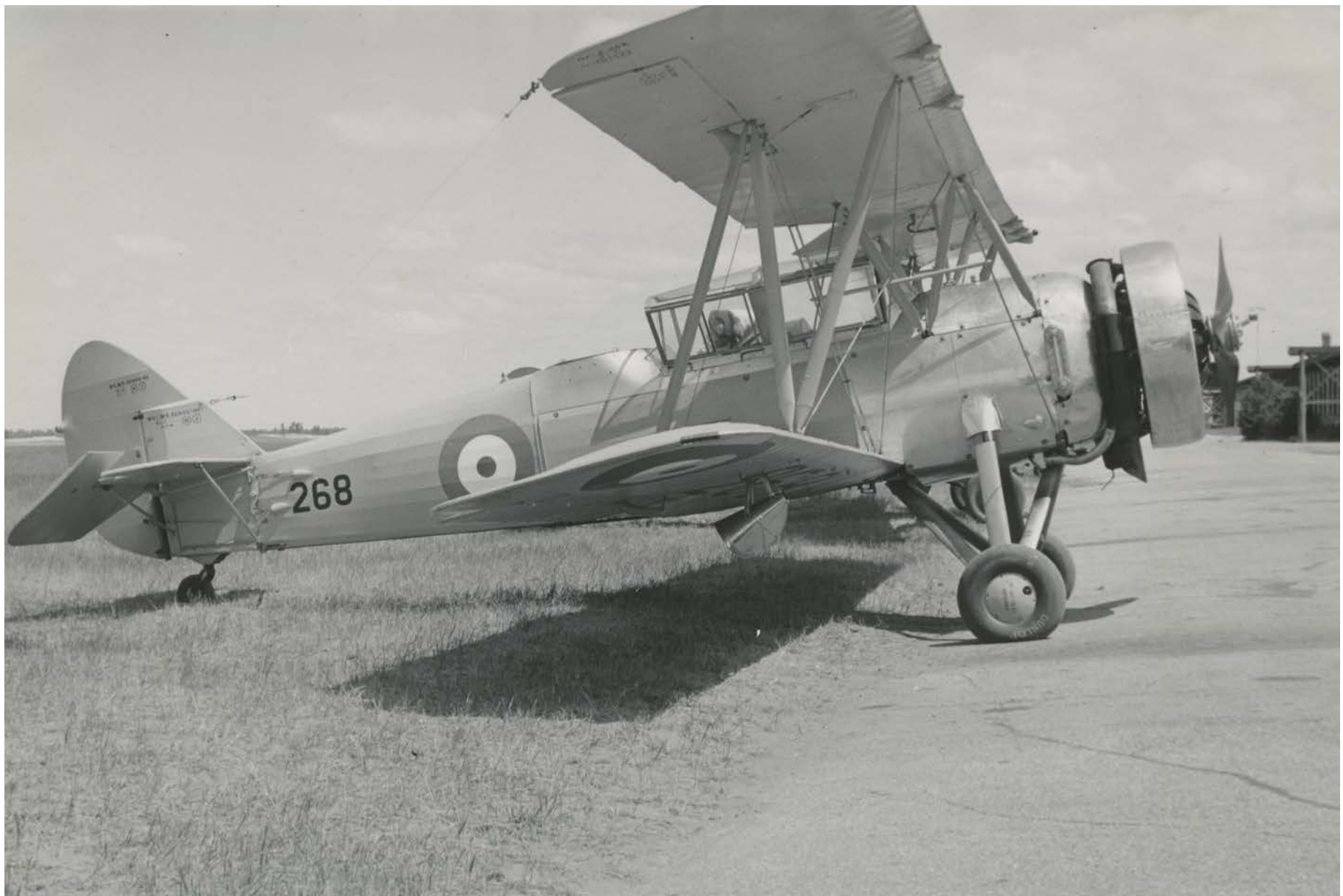
Avro 626 trainer no. 268 is pictured here on the flight line at Camp Borden, Ontario. Note the enclosed cockpit on this A/C. (J. McNulty Collection photo)
