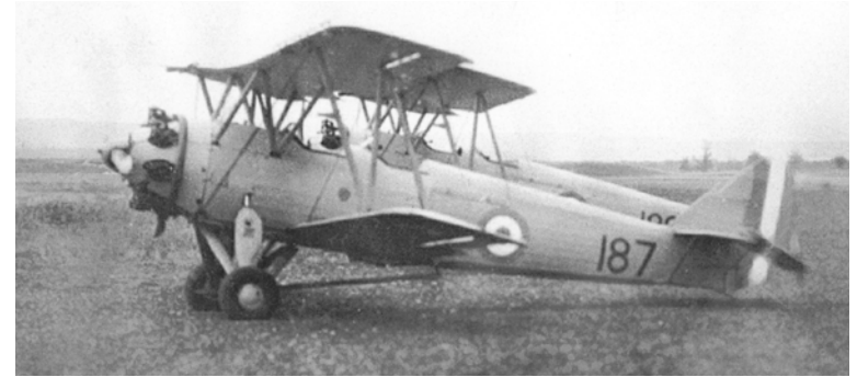
Two RCAF Avro Tutors following conversion to the army cooperation training role, as evidenced by the long hook under the fuselages. (CF photo)
