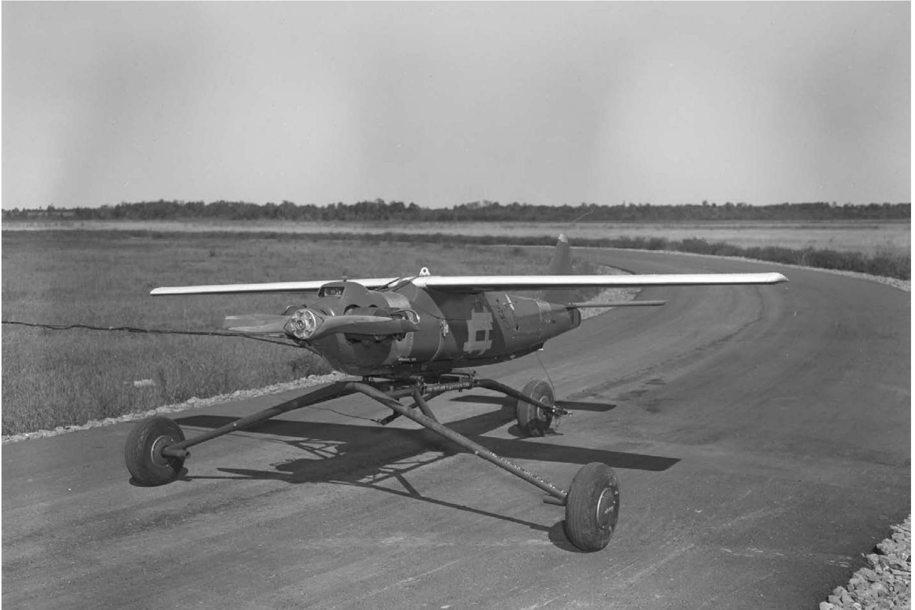
These photos provide three views of the little-known Radioplane OQ-19 target drone being tested by the RCAF. (RCAF photos)
