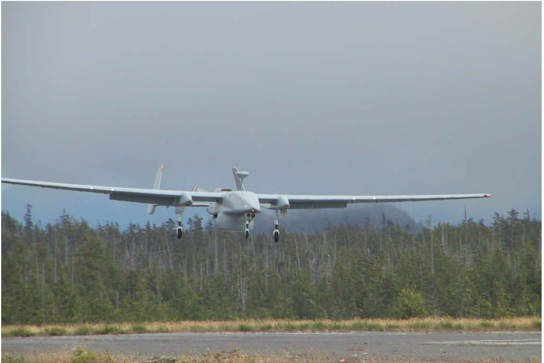
The Eagle UAV, designated CU-160, as leased by the CF. (CF photo)
