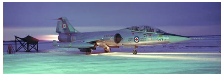
This CF-104D from No. 417 Squadron is having its engine tested in full afterburner. The ensuing roar on a cold winter's night could be heard all over the base. (RCAF photo REC04-1601)
