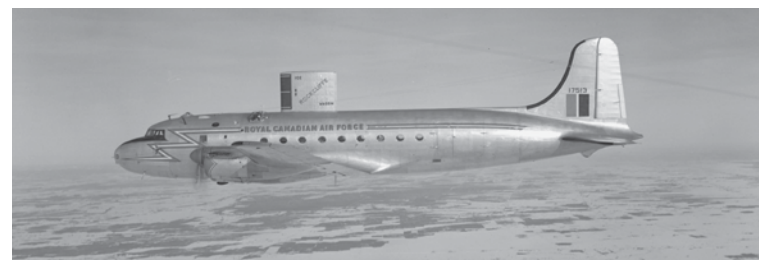
This special North Star aircraft, known as the “Rockcliffe Ice Wagon,” was heavily modified and used for airborne icing research/trials. (RCAF photo PL-53288)
