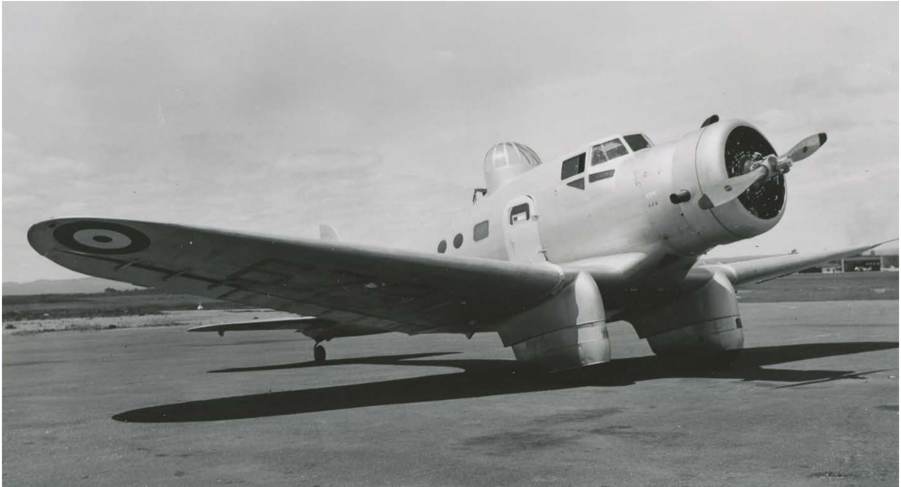
A photo taken in 1939 of an RCAF Northrop Delta Mk II variant complete with the rear dorsal turret. (Photo courtesy of G. L. McNulty Collection)
