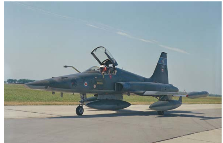
This CF-116A Freedom Fighter illustrates the recce-camera nose that could be fitted to the type. It is also equipped with a fixed air-to-air refuelling probe. (CF photo PCN80-67)
