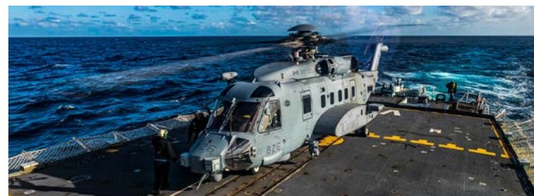
The CH-148 Cyclone uses the same type of "beartrap" landing and takeoff system as its predecessor to allow for operations from heaving ship decks. (CF Combat Camera photo)
