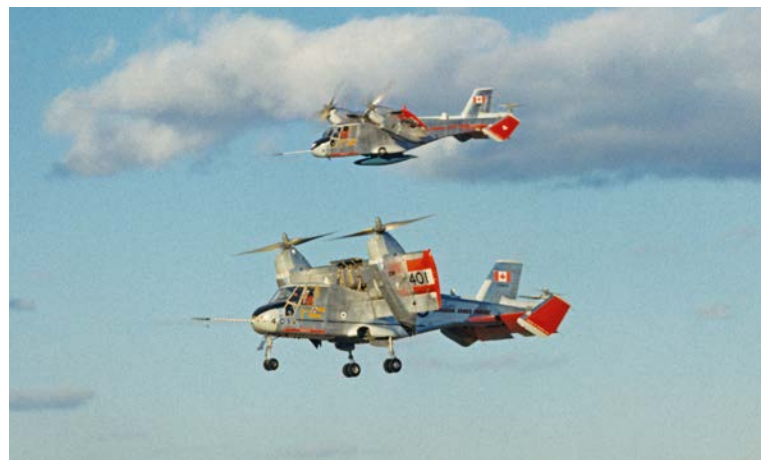
This photo of two Canadair CL-84 Dynaverts in formation illustrates the tiltrotor configuration in action. (Canadair photo)
