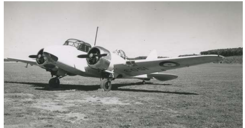
This Airspeed Oxford Mk I no. 1503 has been outfitted for aerial gunnery training. Note the gun turret on the rear of the fuselage. (RCAF photo HC-8704)
