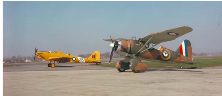
The Fairey Battle gunnery trainer in the background and the Westland Lysander aircraft for target towing in the foreground formed the backbone of the BCATP in the early stages of the programme. In the target-towing role the Lysander was often painted in overall yellow BCATP finish with large black diagonal stripes. (CF photo RNC-1474-5)
