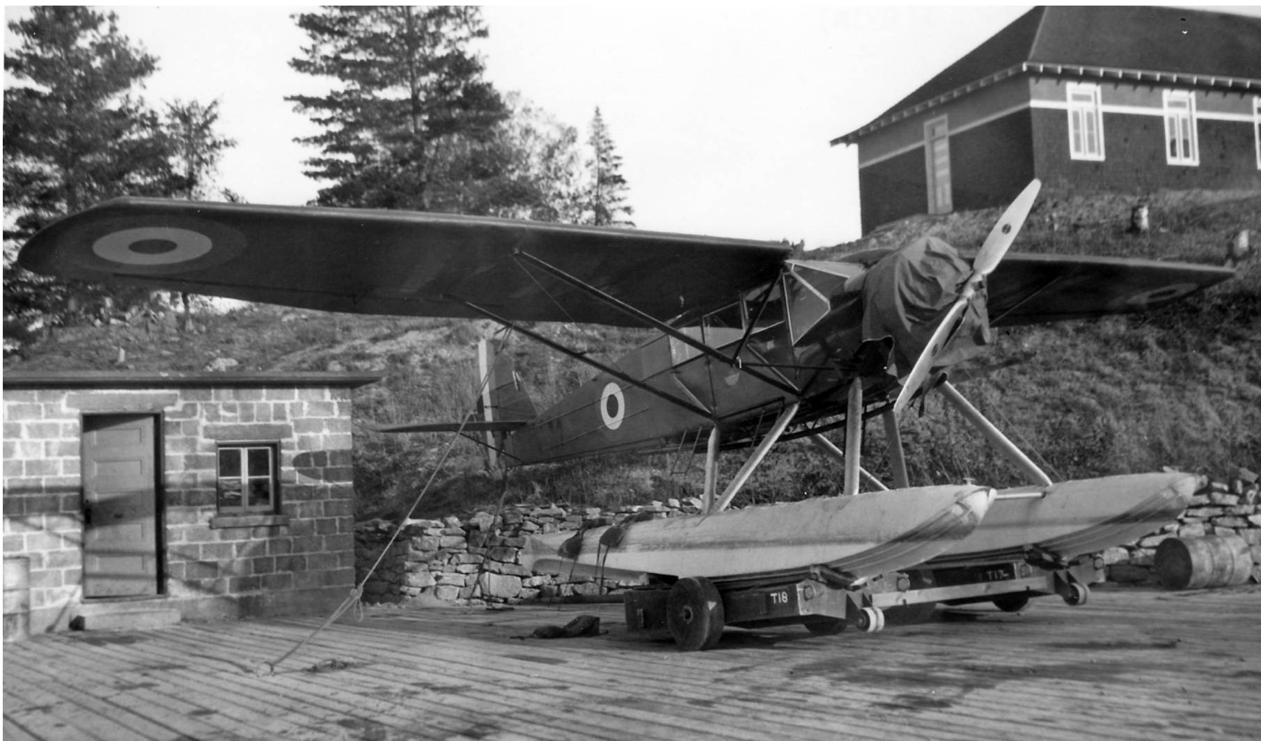
An RCAF De Havilland Hawk Moth in a float-plane configuration is seen here laid up on a beaching dolly. The float-plane configuration revealed structural problems with the design. (Library and Archives Canada photo PA62799)
