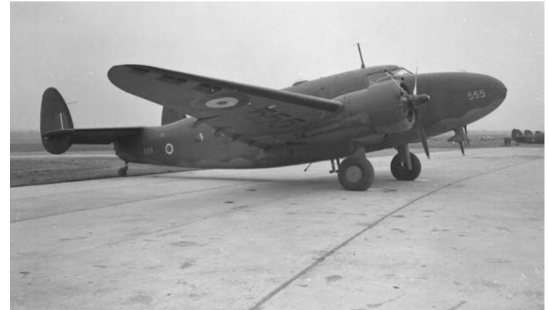
The fully camouflaged RCAF Lockheed Lodestar transport 555 on the tarmac. Towards the end of the war, aircraft such as these were stripped of paint to lessen their weight. (RCAF photo RE881-1)
