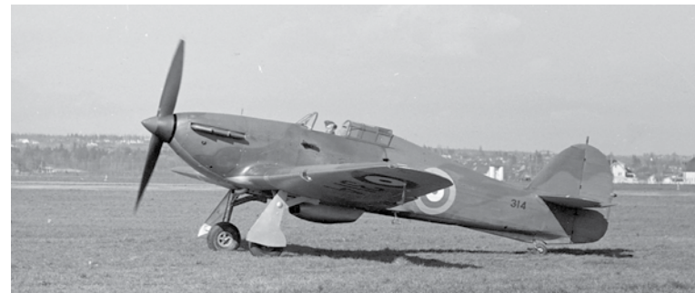
In the photo is an early model Mk I Hurricane in Canada; note the two-bladed propeller. Canada also manufactured Hawker Hurricanes at the Canadian Car and Foundry plant in Ontario. (RCAF photo)
