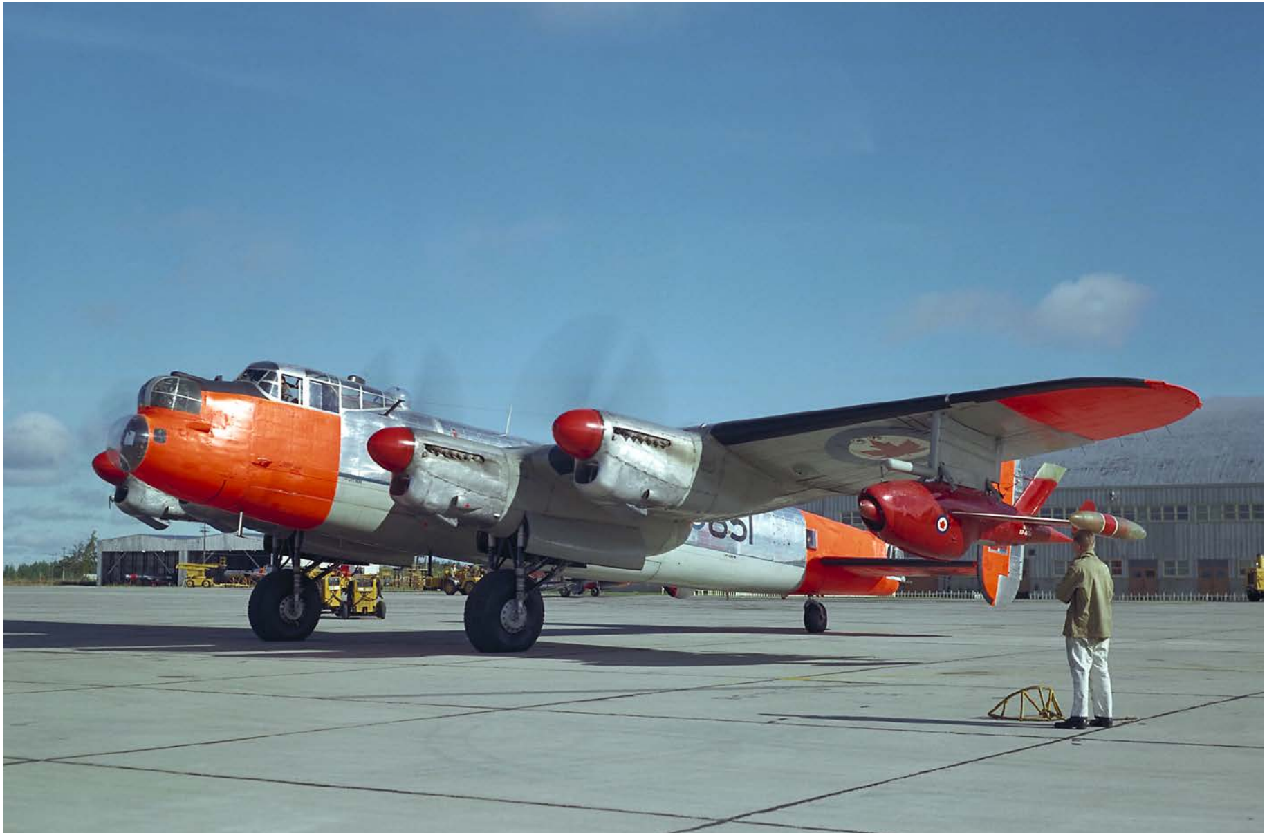
Two RCAF Lancaster Mk 10s were modified as launch and control platforms for Teledyne-Ryan Firebee drones in Canadian service. Recovery of the drones was effected by parachute. Note the mission tally on the Firebee drone in the photo on the opposite page. (RCAF photos PCN-1962)
