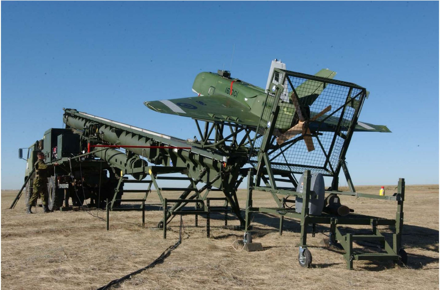
The CU-161 Sperwer UAV along with its launch system as deployed to Op ATHENA in Afghanistan is shown here. (CF photo LT2005-0467d)
