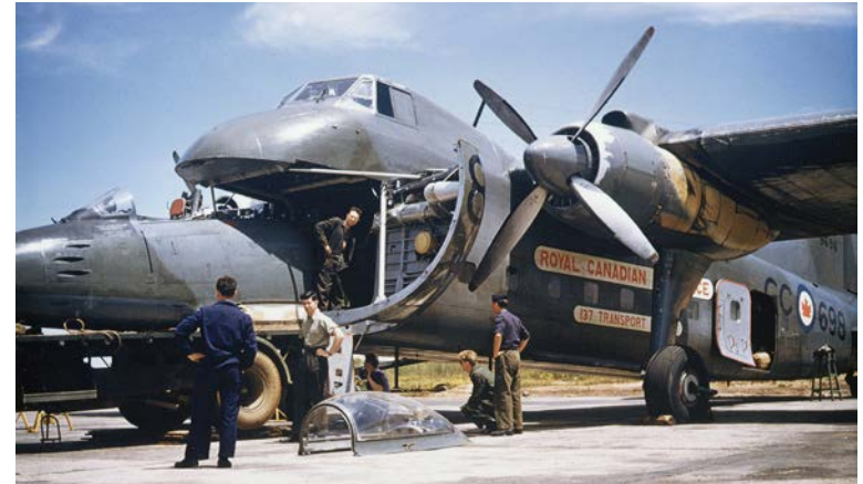
The RCAF Bristol Freighter could carry a dismantled F-86 Sabre from RCAF bases in Europe to repair and overhaul facilities in Prestwick, Scotland. (BCAM photo)
