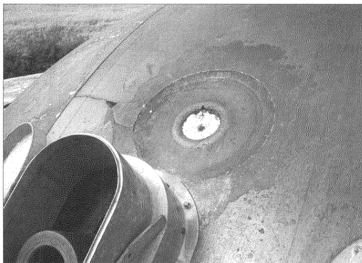
120mm gun cupola with 50kg shaped charge crater.
