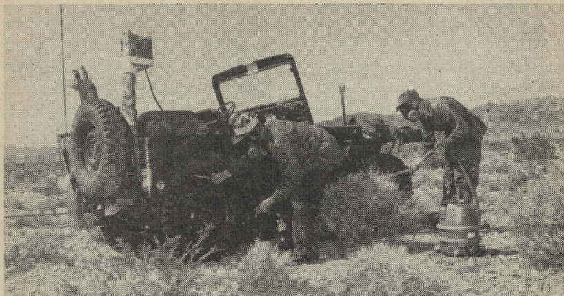
A vehicle which has just returned from a radio-active area is cleaned with a vacuum cleaner or washed with water and then checked with a radiation detector.
