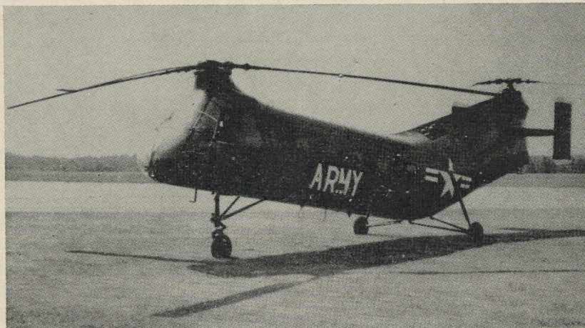
The H-21 light transport helicopter. Typical missions are troop and cargo transport and medical evacuation. Cruise speed is 0-85 knots; range (normal cruise speed), 280 nautical miles; allowable cargo load, 3000 lbs. (40 nautical miles radius), 2200 lbs. (140 nautical miles radius). It has a crew of 3; troop capacity (combat equipped), 12; litter capacity, 12; hours of flight (normal cruise speed, design gross weight), 3½.
