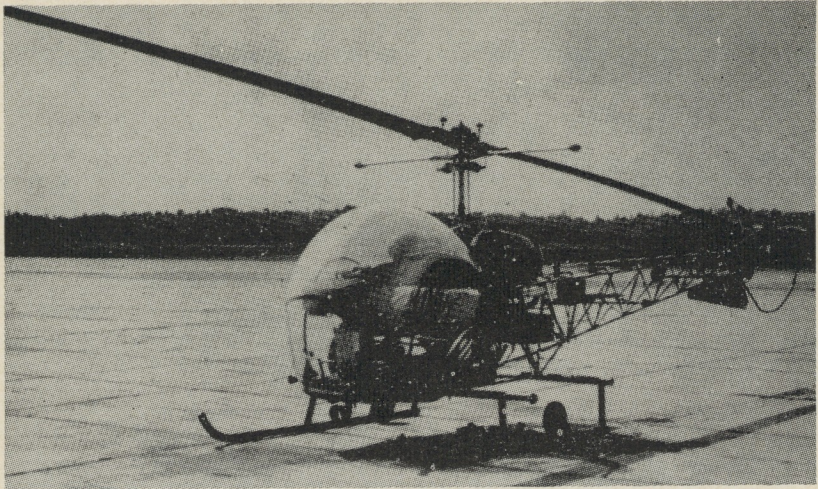
The H-13 reconnaissance helicopter, typical missions of which are observation, medical evacuation, wire laying and command liaison. The cruise speed is 0-70 knots and range (normal cruise speed), 130 nautical miles. The allowable cargo load is 400 lbs.; crew, 1 (pilot); troop capacity (normal cruise speed, normal gross weight), 2; litter capacity, 2; hours of flight (normal cruise speed, normal gross weight), 3.
