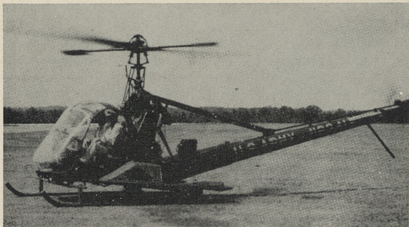
The H-23, another reconnaissance helicopter. Its missions are the same as for the H-13. The cruise speed is 0-60 knots and range (normal cruise speed), 117 nautical miles. Troop capacity (combat equipped) is 2 and litter capacity, 2.
