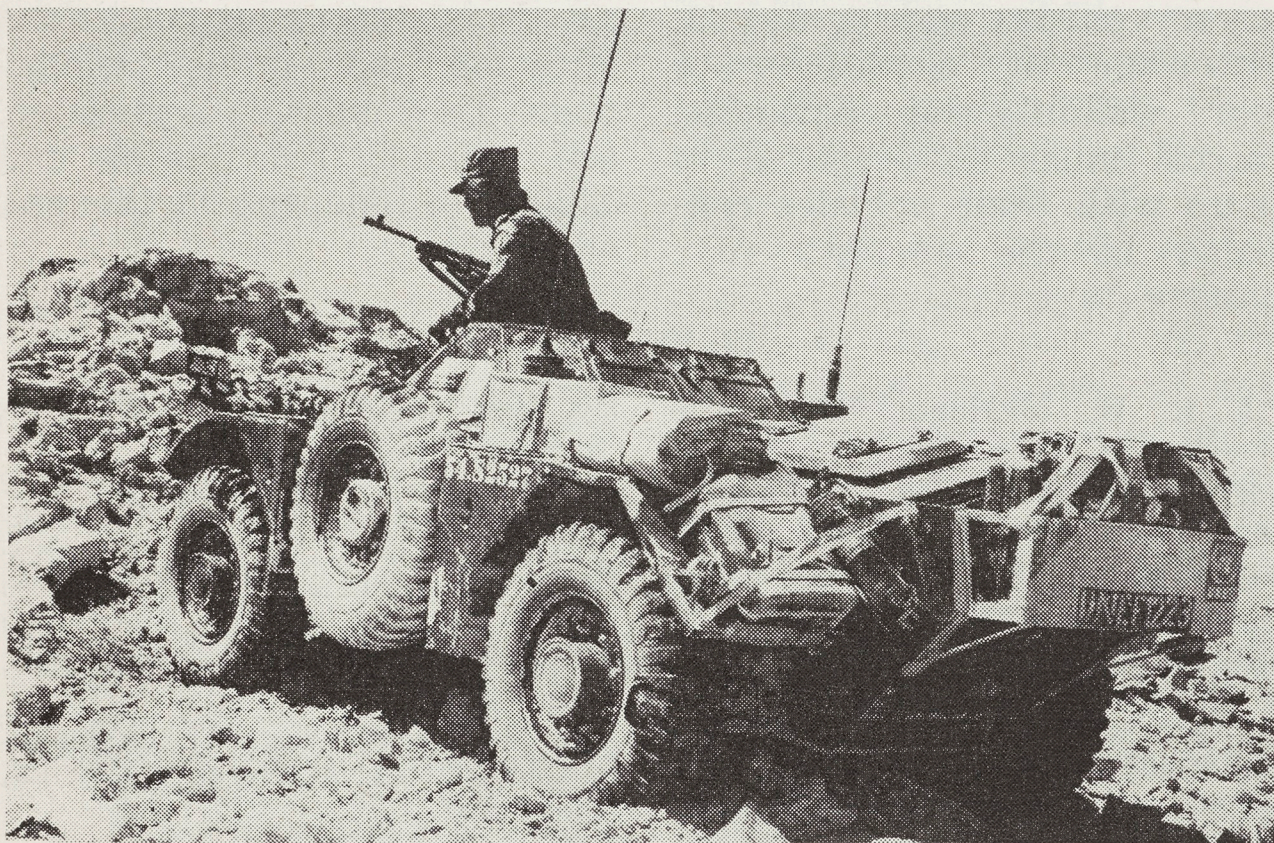
A Ferret Mark I Scout Car of the 56th Canadian Reconnaissance Squadron in the Sinai Desert. This vehicle has been modified to carry extra water cans in a rack at the rear of the engine compartment. It carries a crew of three: one man only is shown in the fighting compartment of this vehicle but provision is made for two. Armament: A light machine-gun and six smoke dischargers.
