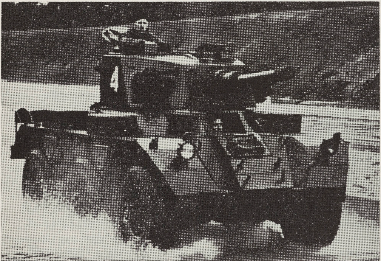
The Saladin, a recent British armoured car which carries a crew of three. Armament: 76-mm. gun and a .30-calibre machine-gun.
