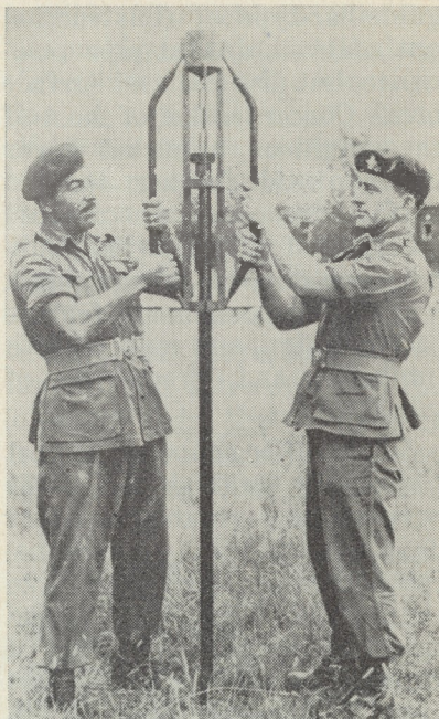
Members of the Royal 22e Régiment using the picket driver on user trials.
