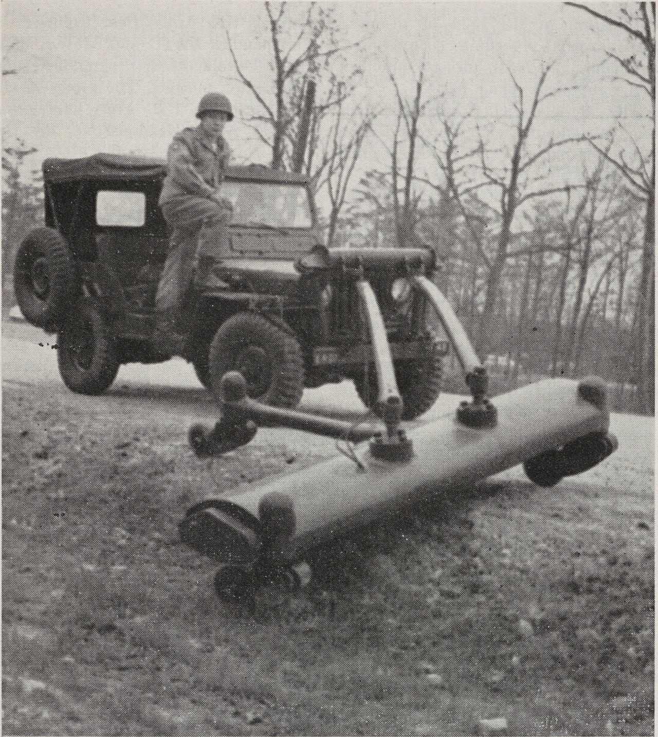
This standardized mine detector can be mounted on vehicles of all three ABC Programme countries.
