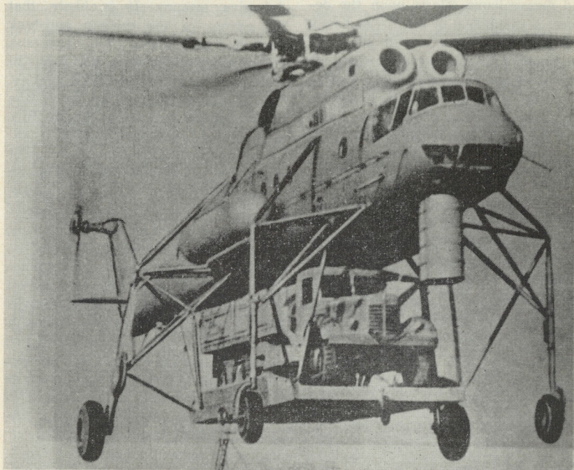
Soviet Mi 10 (HARKE) transport helicopter carrying a 12-ton truck. The maximum payload is 33,302 lbs. or 80 passengers.
