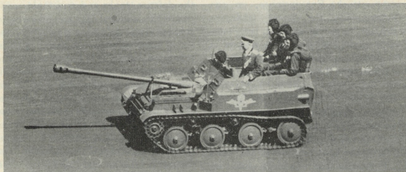
Soviet ASU-57. Weighing six tons, this 57-mm. assault gun can be dropped by parachute. A heavier version mounting an 85-mm. gun is now in service.
