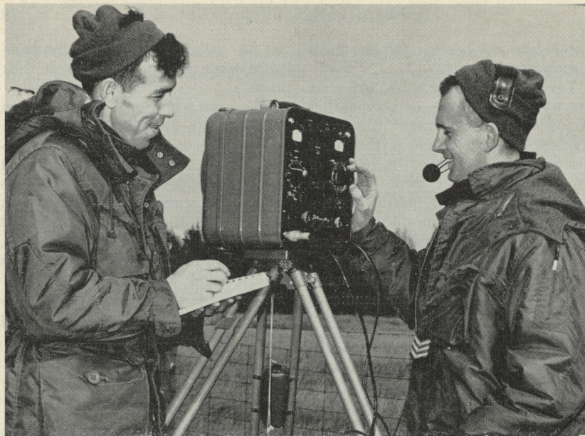
Sergeant R. Hunter, left, and Sergeant E. Tanner, employed in the Army Survey Establishment, Ottawa, are members of the mapping party which operated in Canada's north this past summer. Included in their equipment was this tellurometer, a device which measures distance electronically.
