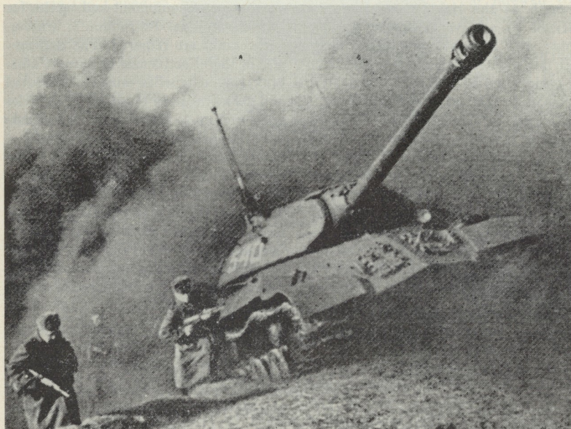
Soviet Joseph Stalin 3. This tank is the predecessor of the T 10, and significant numbers remain in service. The gun is a 122-mm.
