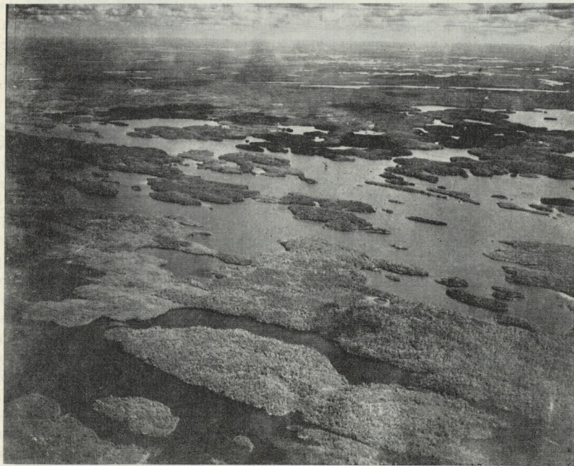
Figure 1: An oblique photograph used for mapping by the perspective grid method
