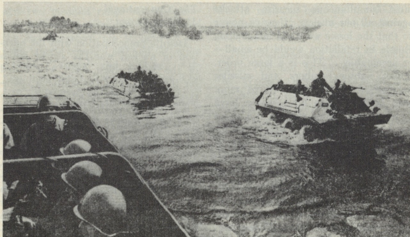
A feature of a Soviet advance would be the rapid passage of water obstacles. This armoured personnel carrier is the eight-wheeled BTR 60p.
