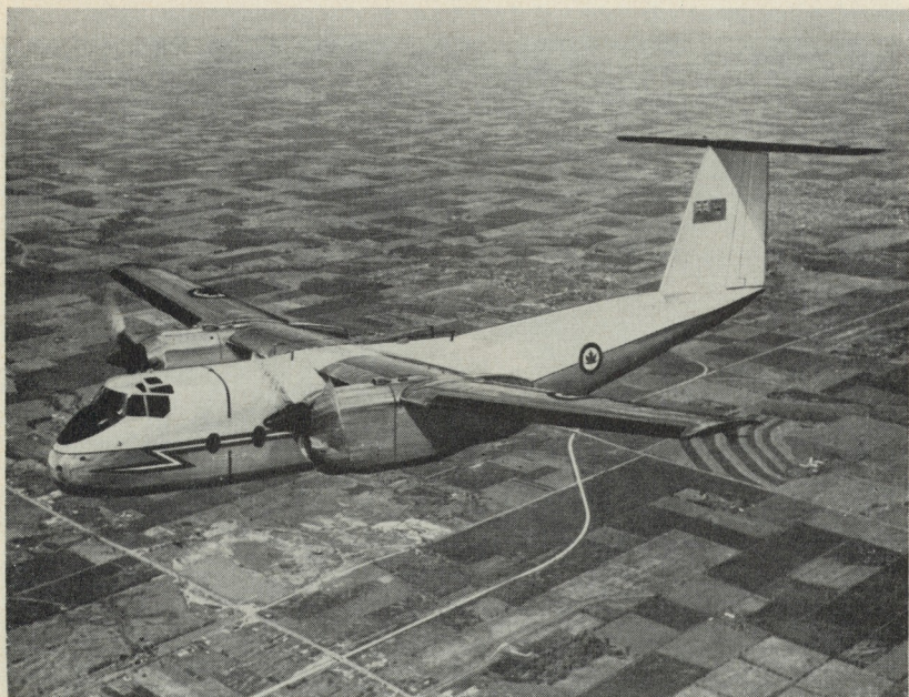
The RCAF's Buffalo . This is a short take-off and landing transport aircraft of medium range with considerable capacity for airlifting either troops or cargo. It is planned to purchase 15 of this type of aircraft.
