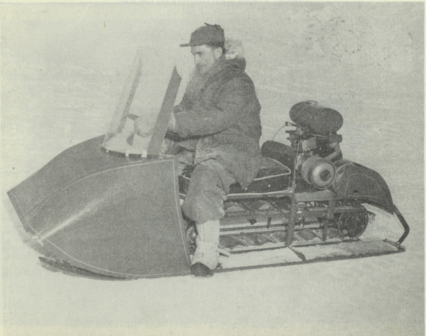
Below: A motor toboggan which is used to tow ground reconnaissance party stores.
