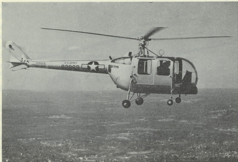
The Sikorsky H-18, a four-place helicopter, is well suited for transporting personnel or cargo.
