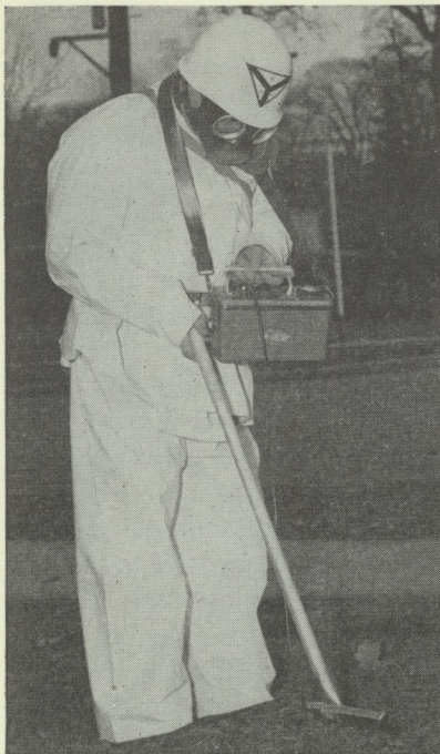
Capt. L. H. Love of 1 RDU checks for atomic radiation during "Exercise Hope". The instrument in his hand is a Geiger counter to measure the amount of radiation present.
