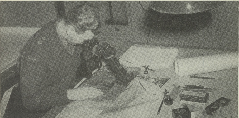
A Canadian officer is shown using a binocular stereoscope to study an aerial photo.
