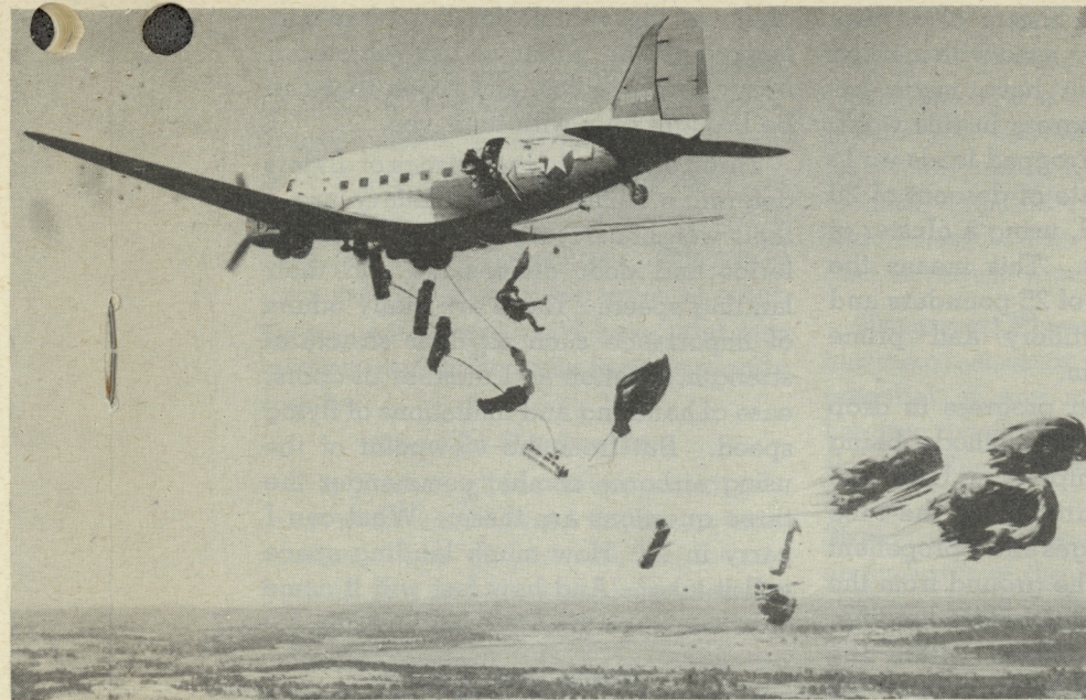
Men and equipment are being dropped from a Dakota. The door loads have been pushed out, and as No. 1 jumper has left the door the para-pack loads have been released. In this case, men and a 75mm pack howitzer with stores and ammunition are being dropped.
