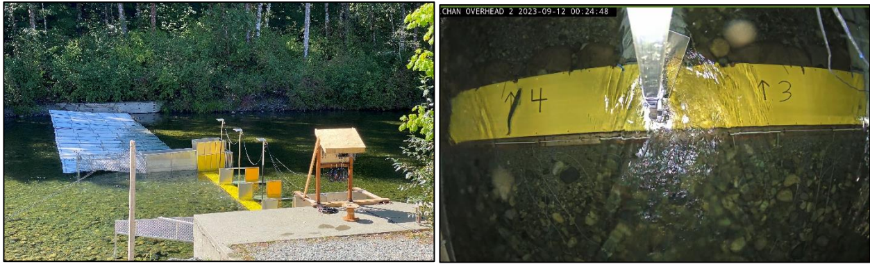
Figure 3: Traditional two-passage counting fence design used since 2019 (top) compared to the new low-flow design with four open passageways and overhead camera views (bottom).
