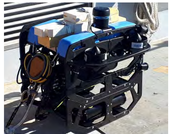
Image 2: "Blue ROV2" used to survey anchorage sites.
