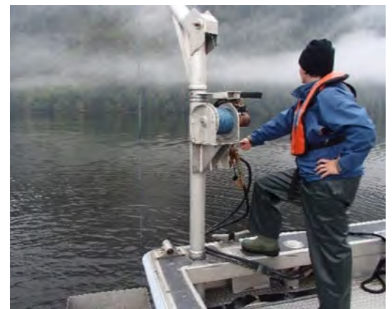
Image 2: Deploying a Van Veen grab for benthic sampling.
