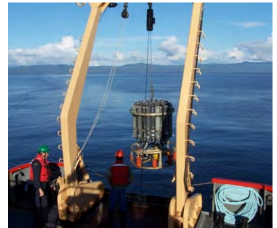
Image 2: Deployment of a rosette, a deep water sampling apparatus. Credit: Fisheries and Oceans Canada
