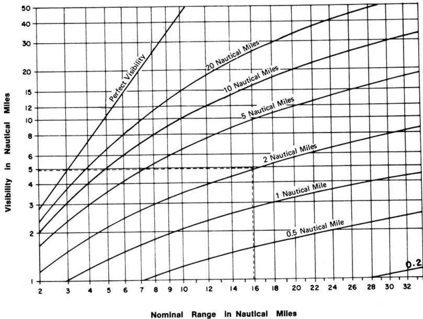
The light list in column 7 gives the nominal range of each lightstation optic where there is sufficient light to be seen 2 nautical miles or more when the meteorological visibility is 10 nautical miles.
