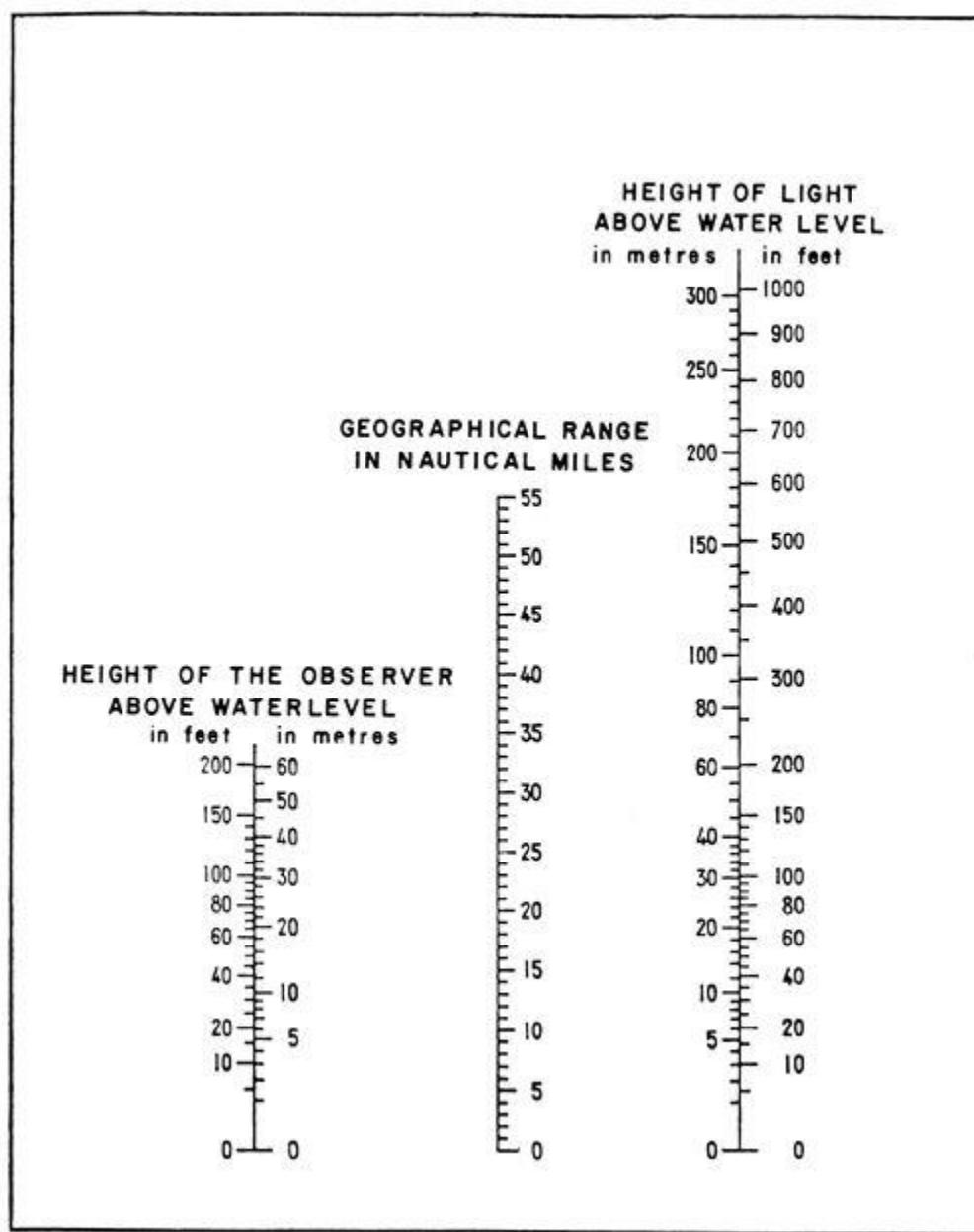
By using the above Nomogram a geographical range can be determined by placing a straightedge against the height of the respective light and the height of the observer above water level.
