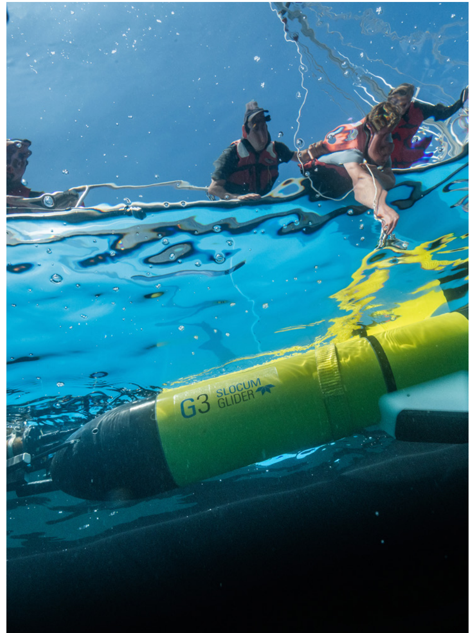
The Ocean Tracking Network (OTN) deploys an autonomous glider off Halifax, Nova Scotia. The gliders provide oceanographic data and record the presence of North Atlantic Right Whales by listening for their vocalizations. This information helps researchers to understand changing oceanic conditions and whale behaviours. Nick Hawkins.
