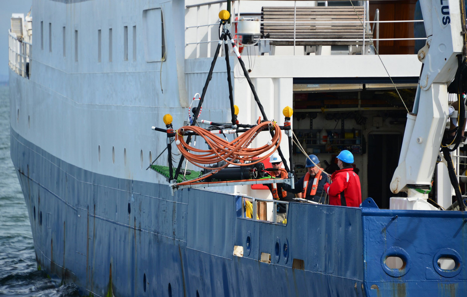
Deployment of hydrophone listening station off the exploration vessel Nautilus. Credit: Ocean Networks Canada.
