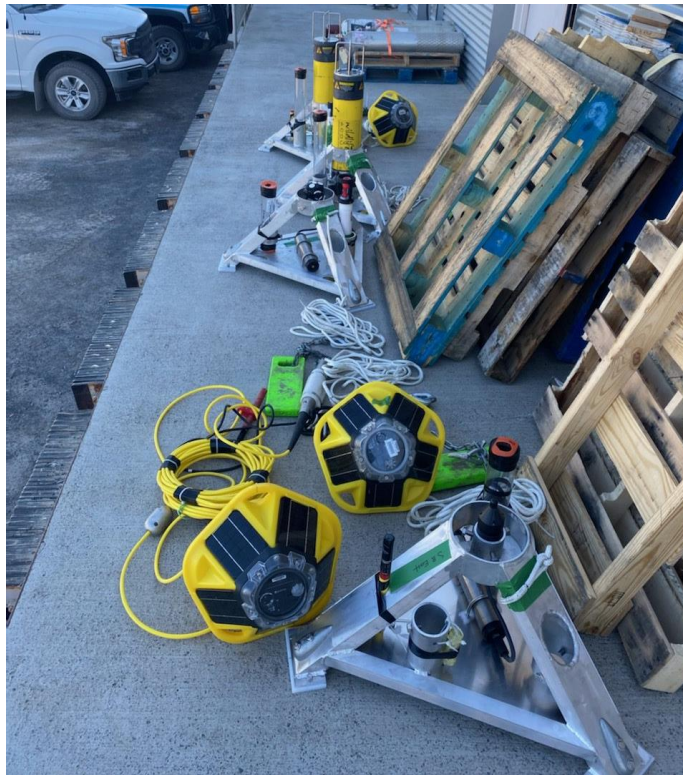
Figure 13: Mooring frames used in 2021 and 2022. Frames equipped with Sound Trap hydrophones are in the foreground, while those equipped with SM2M hydrophones are in the background. Also shown are the 'smart' buoy system.
