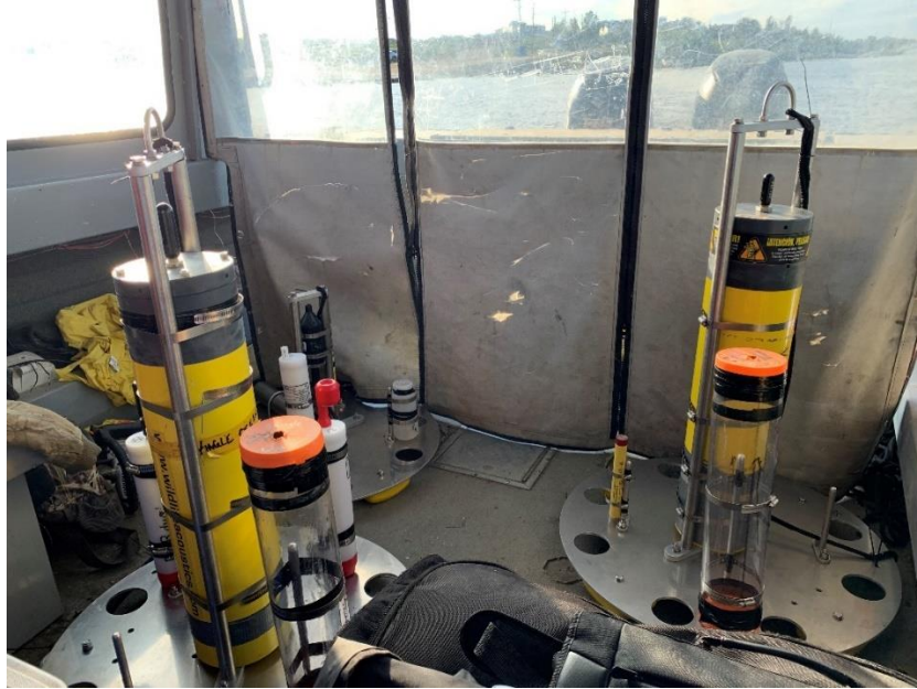
Figure 12: Mooring design in 2020. Two moorings with SM2M acoustic recorders are in front, a smaller mooring with a Sound Trap acoustic recorder is shown in the back.
