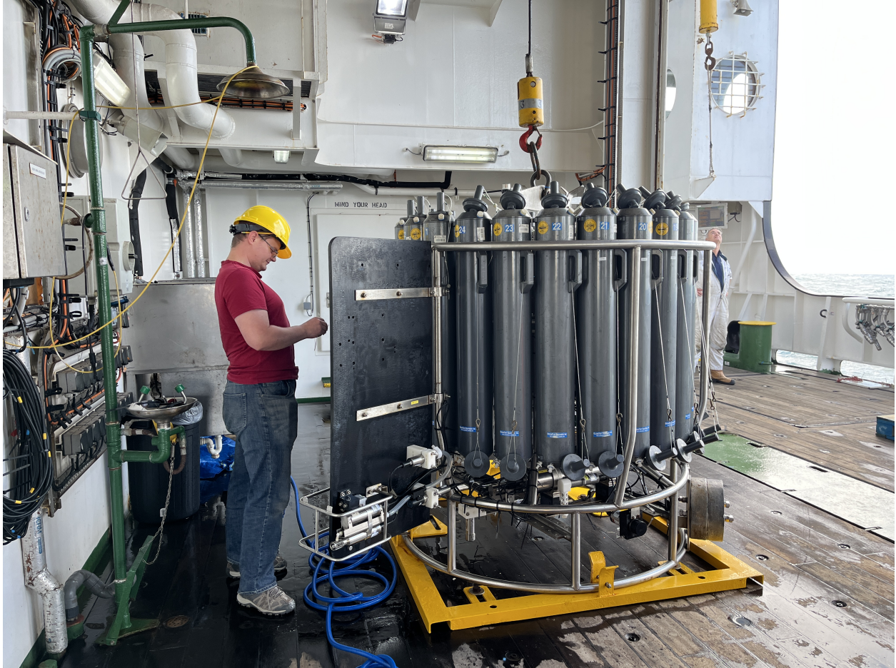
Figure 2. SeaBird (SBE) 24-bottle CTD-Rosette system used during the fall AZMP mission (DY16902). CTD computer operator Patrick Upson is pictured here labelling the Niskin bottles. The CTD was deployed from the starboard deck of the RRS Discovery using the ship's P-frame.
