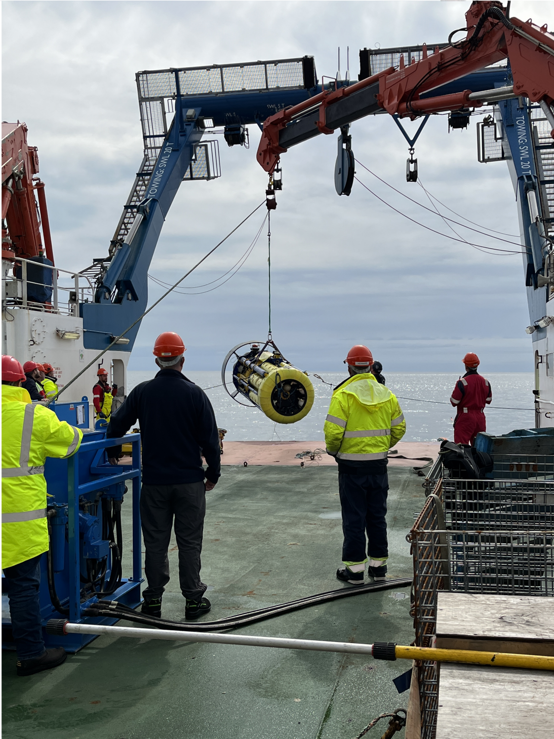
Figure 5. Recovery of the Dalhousie University SeaCycler mechanical float ('mechfloat') using the port-side pedestal crane and mooring winch. The mechfloat was docked in a custom cradle and secured on deck for the remainder of the DY16902 mission.
