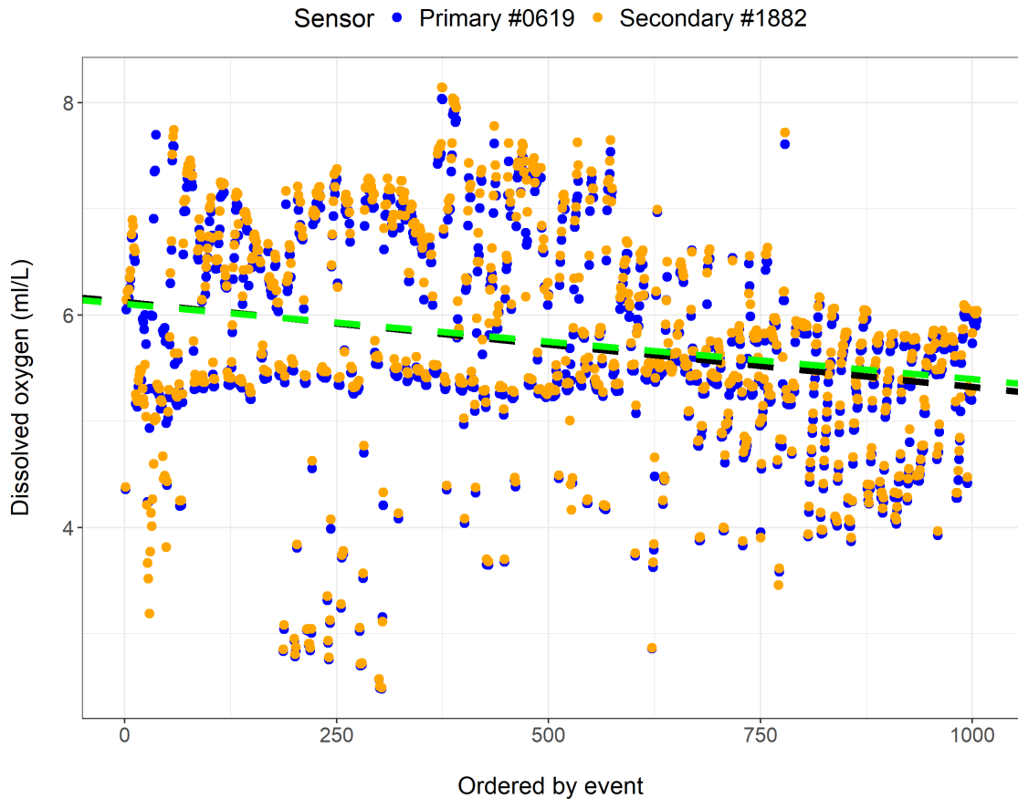
Figure B.1. Comparison of raw primary and secondary dissolved oxygen sensor values for CTD casts collected during the 2023 fall AZMP mission (DY16902). Dashed lines represent the regression between sensor values and sample ID for the primary (blue) and secondary (orange) sensors, respectively.
