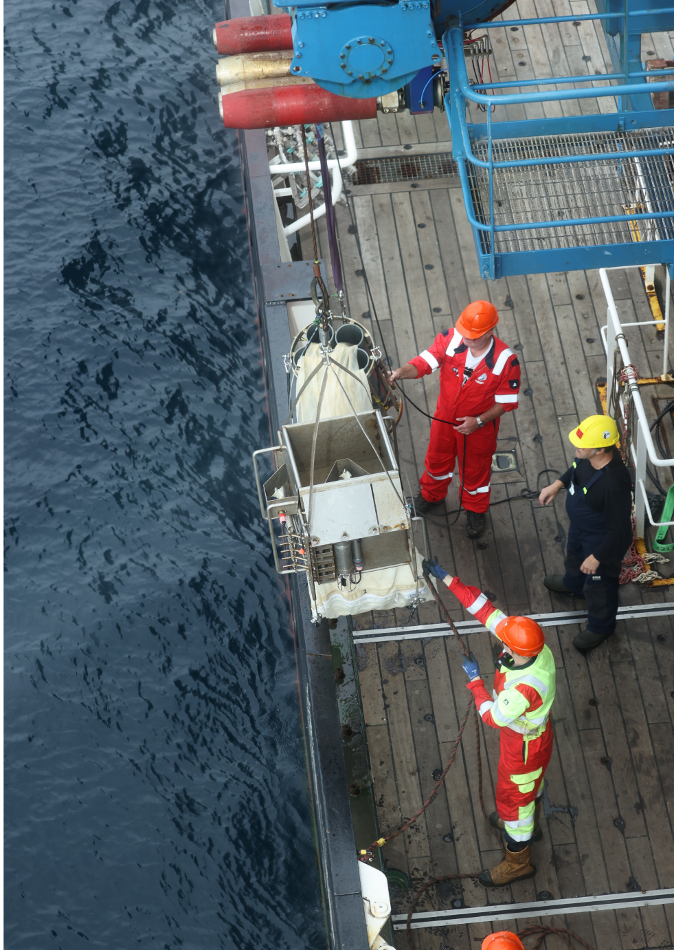
Figure 4. Multinet sampling system used to collect stratified zooplankton samples during the DY16902 mission. An auxiliary winch on the bullhorn boom was used to lift the cod end over the rail.
