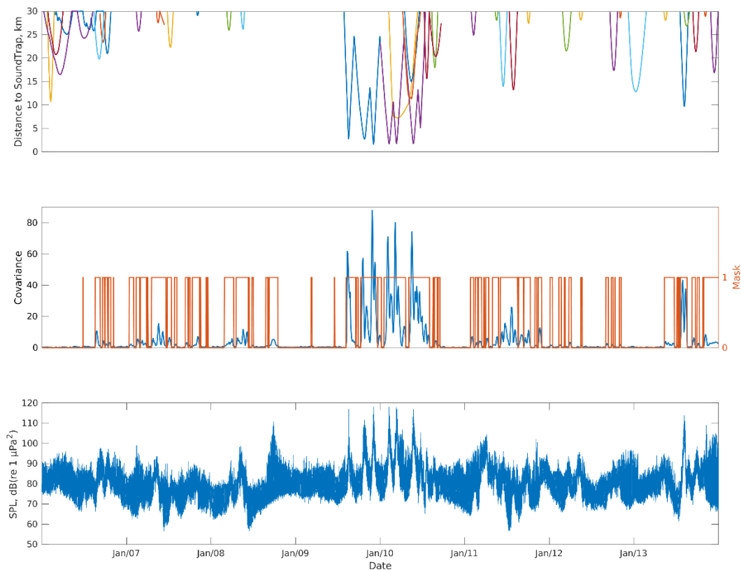
Figure 3. A typical figure used to evaluate the performance of the vessel noise detector. The time period shown for all panels is from January 6 to 14, 2020 (UTC). Top panel: The distance (km) of vessels, travelling at speeds of 1 knot or faster, from the mooring location (30 second resolution); Middle panel: The covariance between noise levels in the 1/3 octave bands centered at 100 and 500 Hz (blue line) and mask values (orange line) resulting from the vessel noise detector (5 minute resolution, mask value of 1 indicates the presence of vessel noise); Bottom panel: The sound pressure level (SPL) in the 1/3 octave band centered at 100 Hz ( 0.3413 second resolution).
