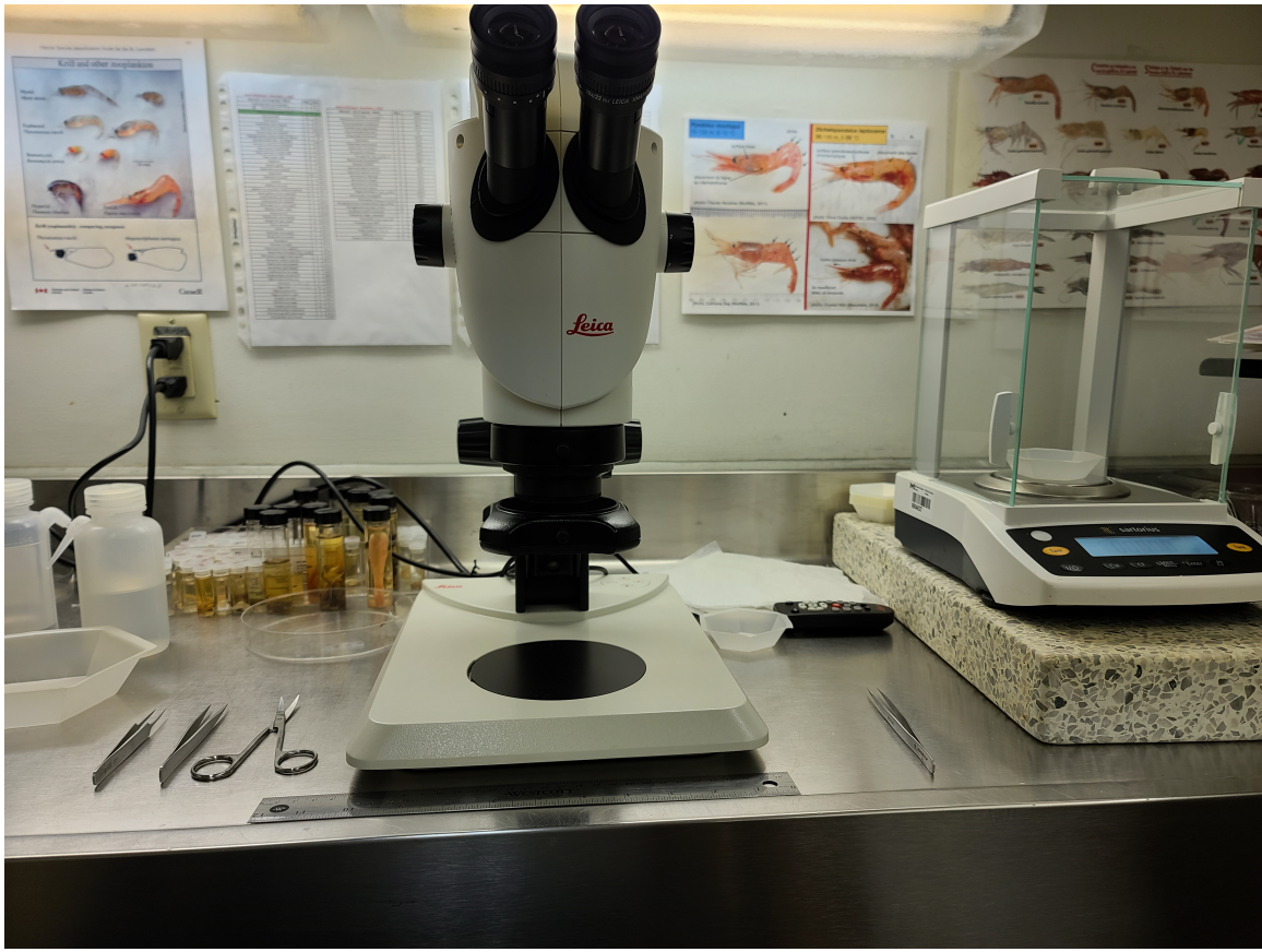
Figure 1. Laboratory configuration to conduct detailed stomach content identification. This setup uses the Leica S9i microscope (6.1x to 55x) with a digital imaging head and a \pm 0.0001\text{g} digital scale.
