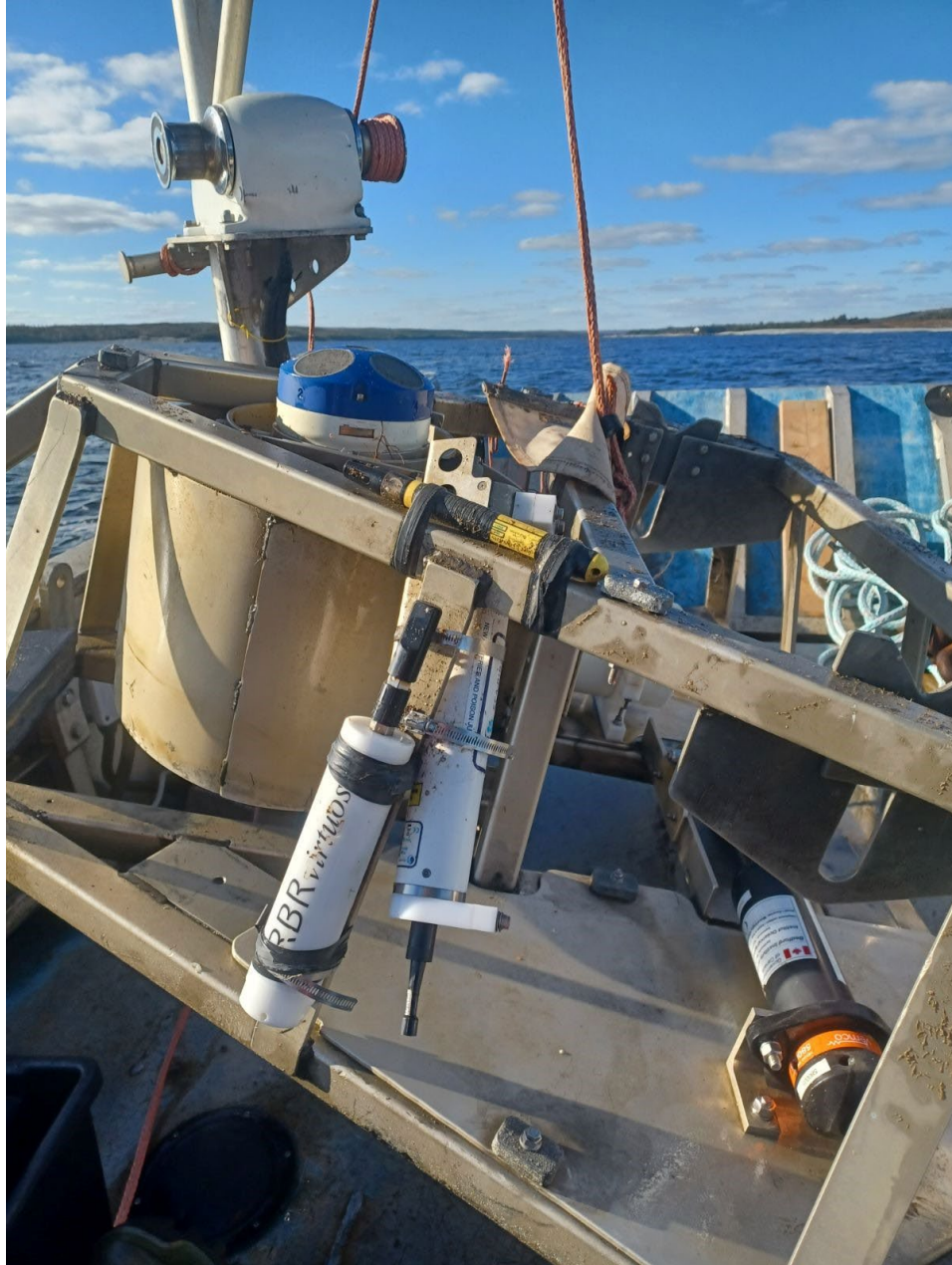
Figure 18. Picture of the ADCP bottom mounted frame place at station ADCP SMR just offshore of the mouth of St. Mary's River estuary. The blue top instrument is the ADCP. The Tu sensor is pointed vertical in white with RBR Virtuoso written on the pressure case. The small horizontal yellow instrument on the top bar of the ADCP frame is the RBR Duet TD wave gauge.
