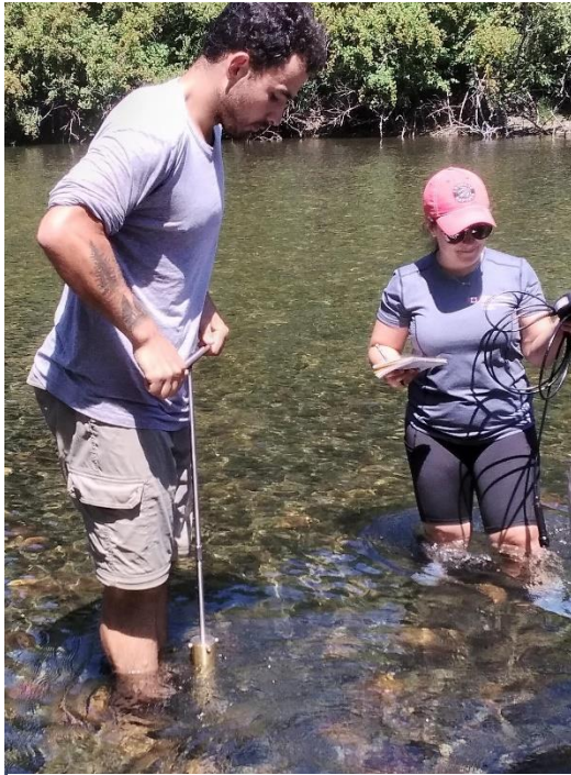
Figure 27. Taking subgravel water sample for oxygen measurement
