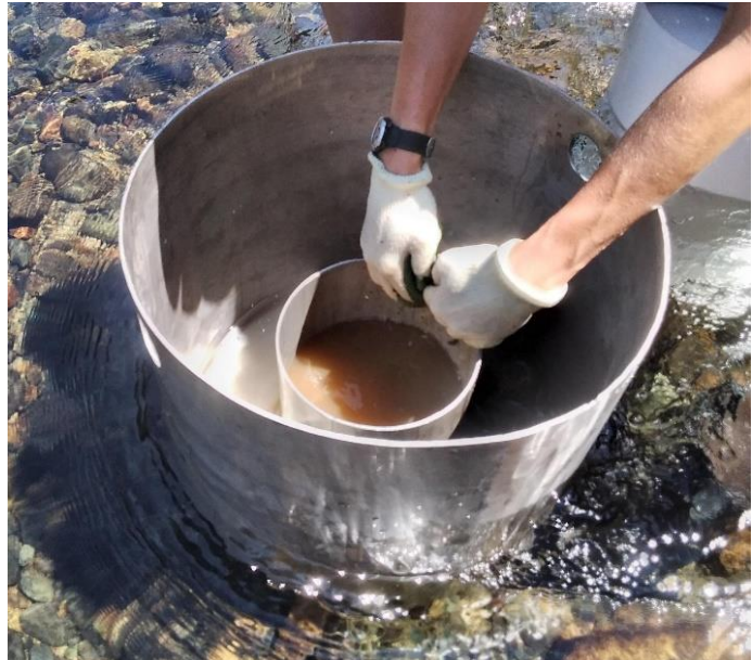
Figure 26. McNeil gravel sampler
