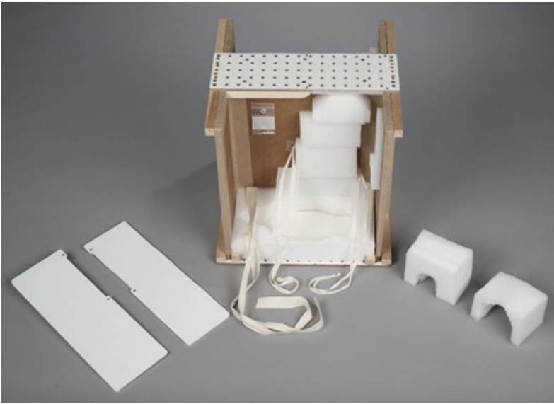
© Government of Canada, Canadian Conservation Institute. 127495-0142 Figure 7a. Items required to build a restraint system for two ceramic dog sculptures separated by a triwall corrugated partition.
