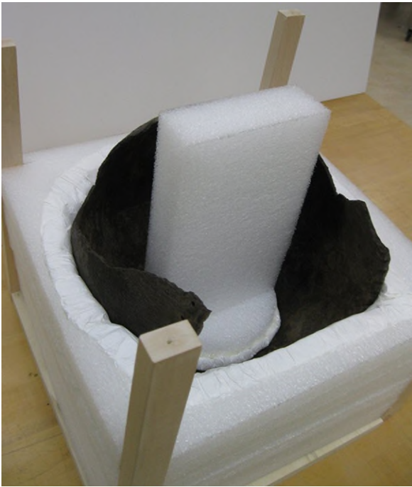
© Government of Canada, Canadian Conservation Institute. 126653-0116 Figure 5b. A polyethylene foam insert with closely conforming base profile and a surface covered in polyester and Tyvek.
