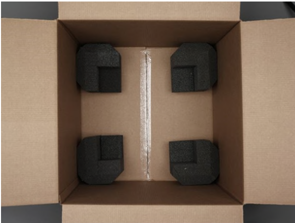
© Government of Canada, Canadian Conservation Institute. 127495-0128 Figure 9a. Bottom corner pads set inside the outer box.
