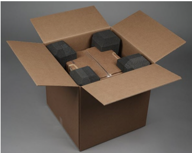
© Government of Canada, Canadian Conservation Institute. 127495-0125 Figure 9b. The inner box floating on eight corner pads before closure of the outer box.
