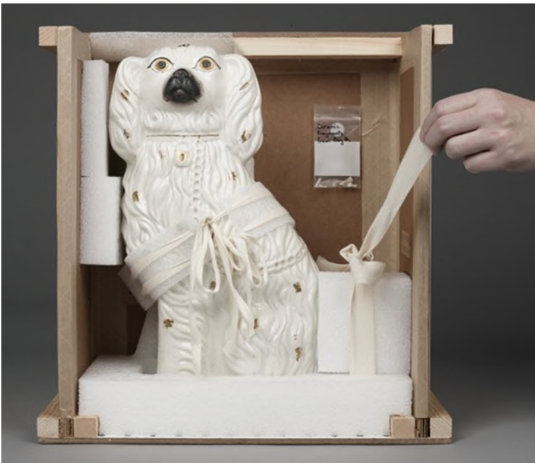
© Government of Canada, Canadian Conservation Institute. 127495-0135 Figure 7b. The dog sculpture restraint on one side of the partition. White foam is firm polyethylene (such as Ethafoam 220).
